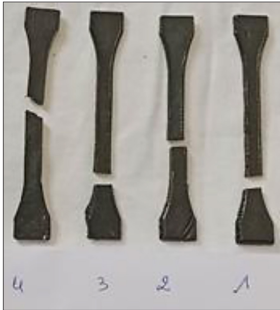
Figure 6. PLA specimens after tensile tests
