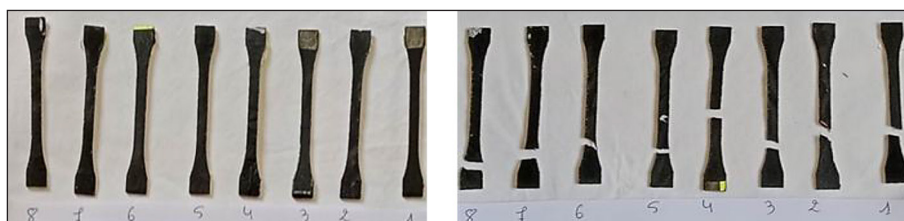
Figure 9. Specimens before and after tensile tests
