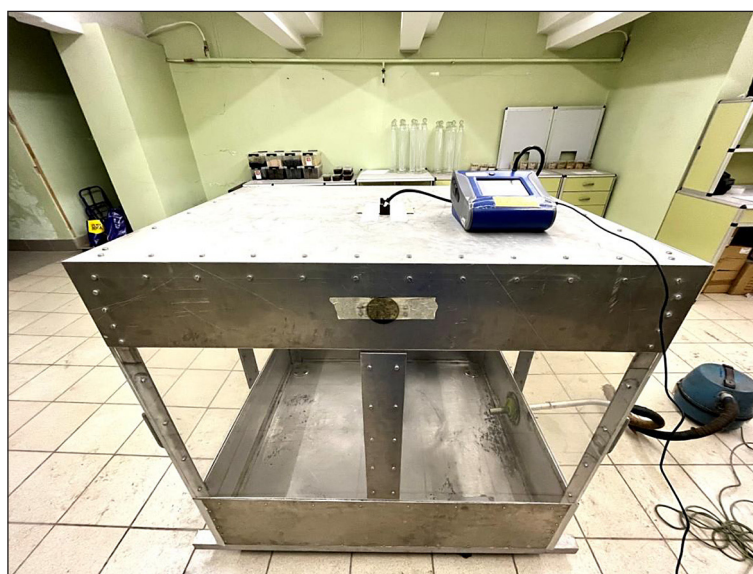
Figure 2. Dust suppression bunker “BPP 001”
