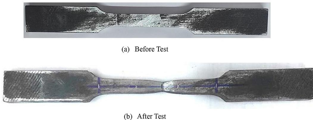
**Figure 1.** Tensile test specimens
