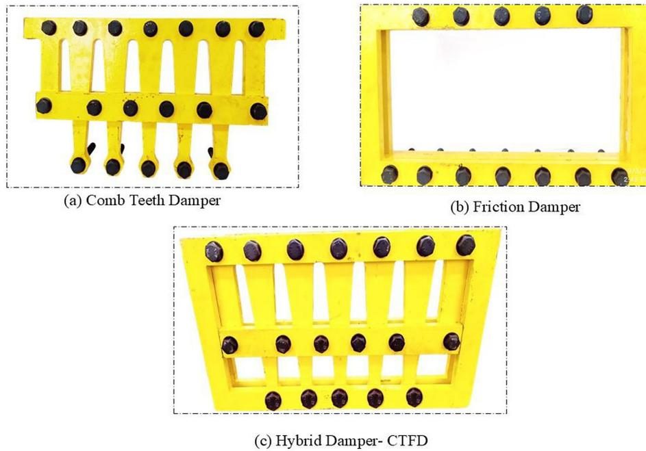
Figure 6. Parts of hybrid damper and assembled CTFD
