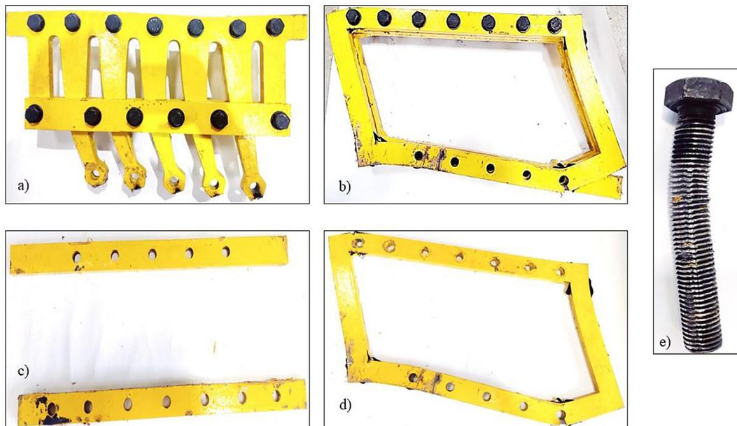
Figure 8. (a) Yielded CTD, (b) failed FD, (c) inner plates of FD, (d) outer plate of FD, (e) failed bolt
