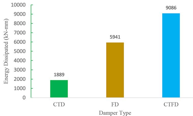
Figure 13. Energy dissipated of FD, CTD, hybrid damper
