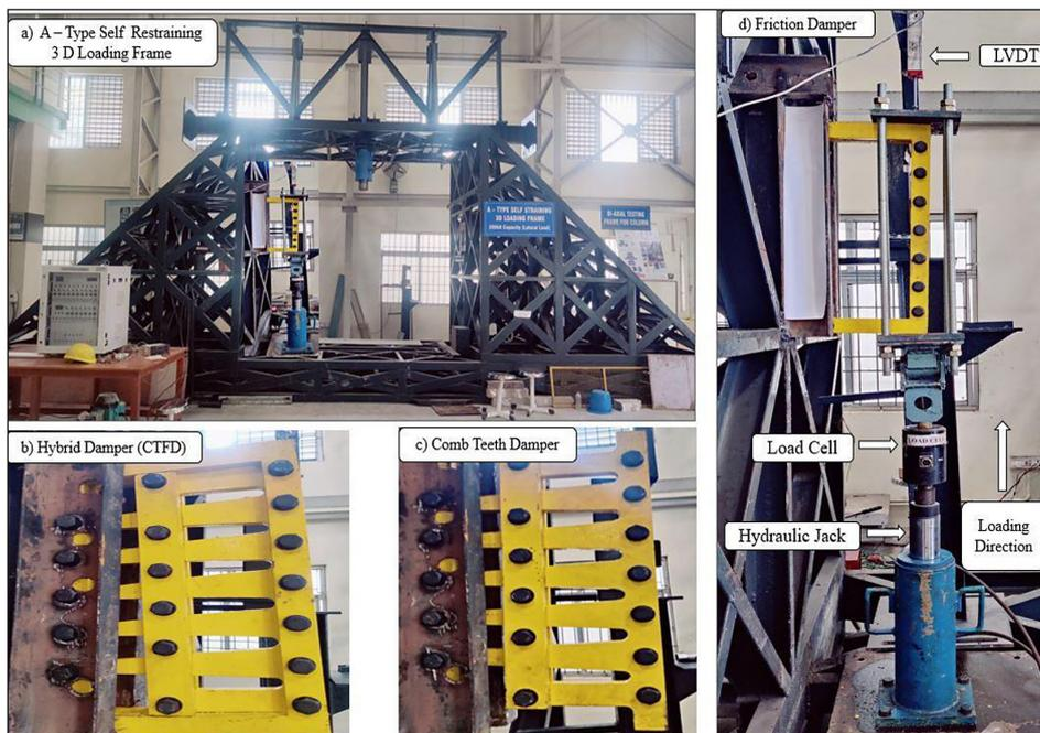
Figure 7. Experimental setup of CTD, FD and CTFD
