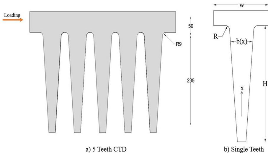
Figure 3. Comb teeth damper -typical & variables of CTD
