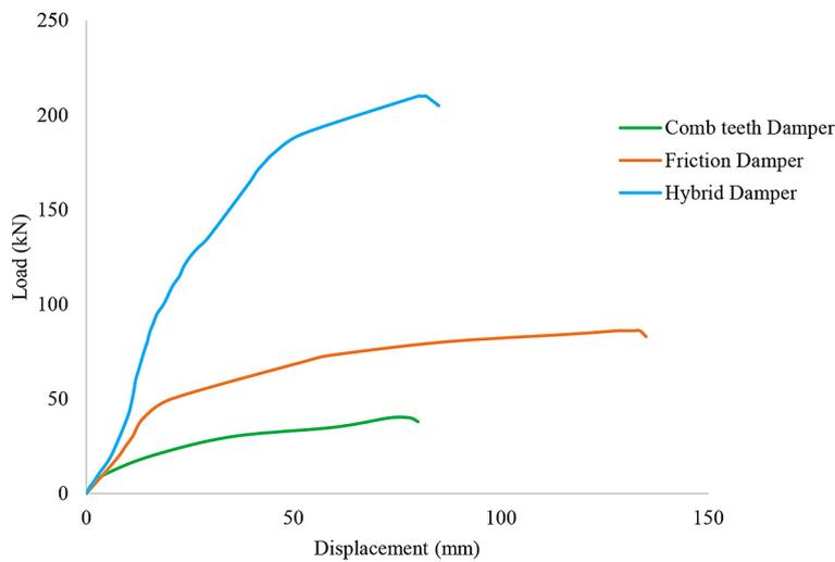
**Figure 10.** Load vs displacement of CTD, FD and CTFD
