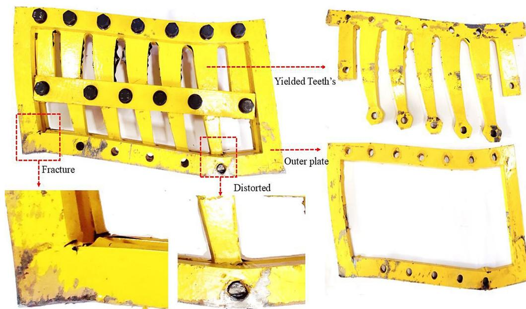
Figure 9. Hybrid damper (CTFD) after failure
