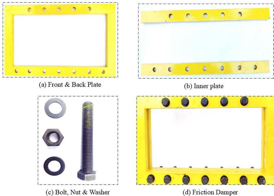
**Figure 5.** Parts of friction damper and assembled FD
