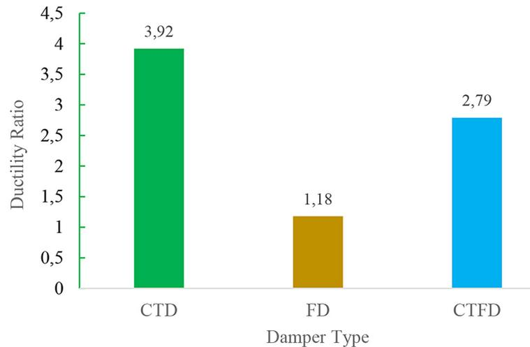
Figure 12. Ductility ratio of FD, CTD, hybrid damper
