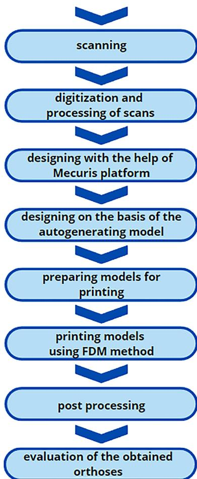
Figure 1. Diagram of work steps
