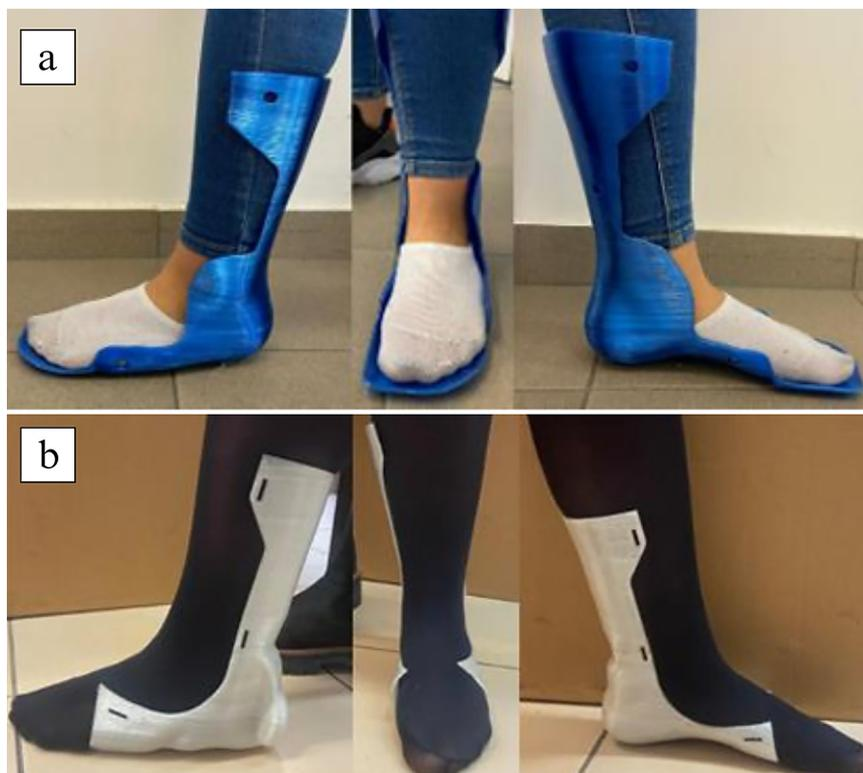
**Figure 14.** Printed orthoses: (a) Mecuris; (b) Inventor
