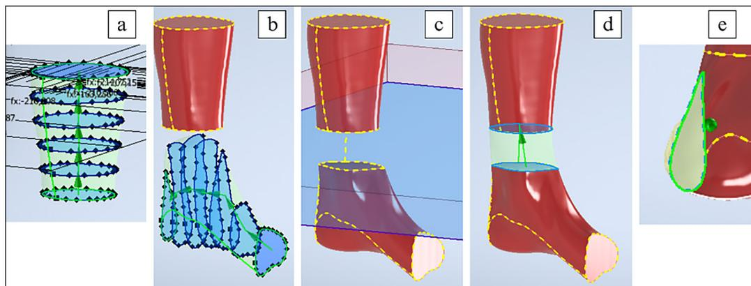
**Figure 8.** Steps to create a model in inventor: (a) view of the planes forming the calf; (b) view of the planes forming the foot; (c) calf and foot with overlapping parts cut out; (d) view of the direction of joining solids; (e) view of attaching the heel
