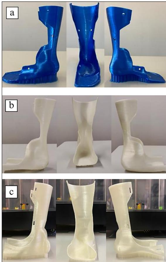
**Figure 13.** Orthosis Printout: (a) No. 2 from Mecuris; (b) No. 3 from Mecuris; (c) No. 2a from Inventor
