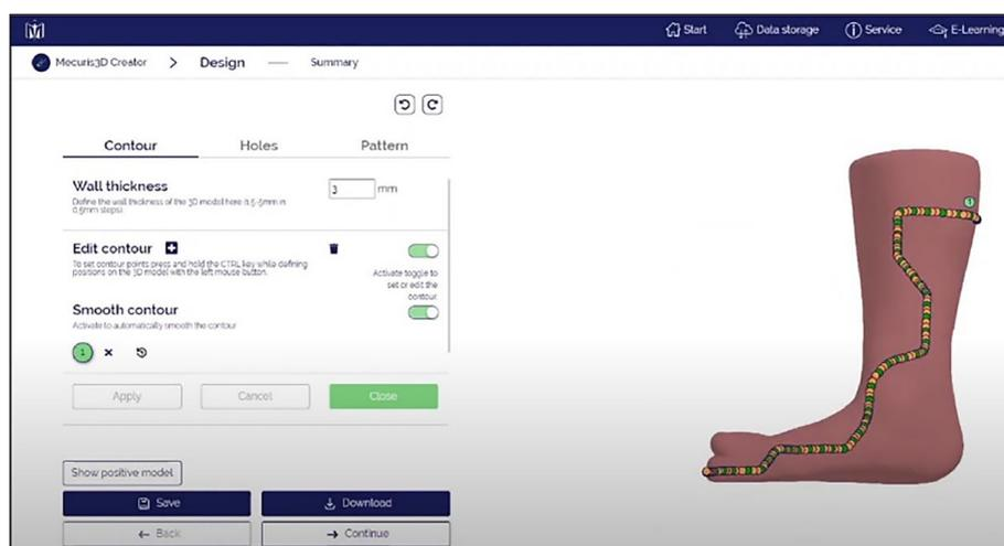
Figure 2. Representation of an orthosis contour consisting of a chain of single points
