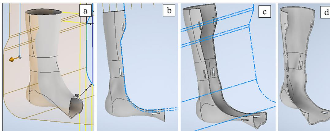
**Figure 9.** Diagram of cutting out the orthosis from the leg model: (a) model shell; (b, c) cutting line of the model from two different perspectives; (d) orthosis model
