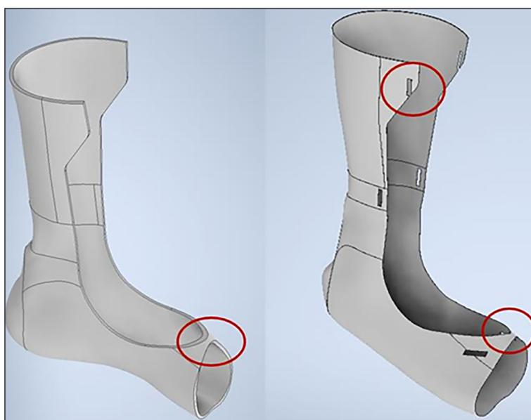
Figure 16. Disadvantages of the autogenerated model without making adjustments
