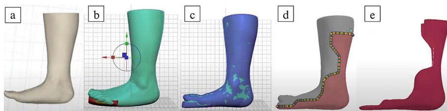
Figure 5. Steps of the design procedure using Mecuris: (a) setting the foot in the normal position; (b) adding an offset and an extension; (c) merging into one solid; (d) determining the cutting line; (e) separating the model along the cutting line
