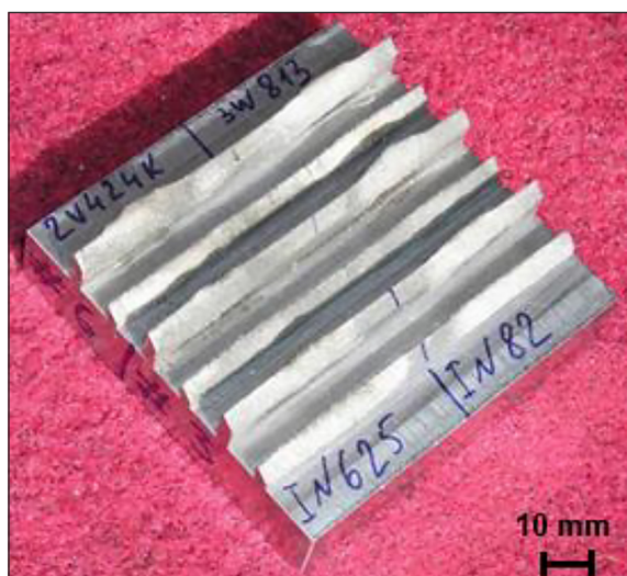
Figure 7. Appearance of a sample with defective zones, restored by microplasma wire spraying
