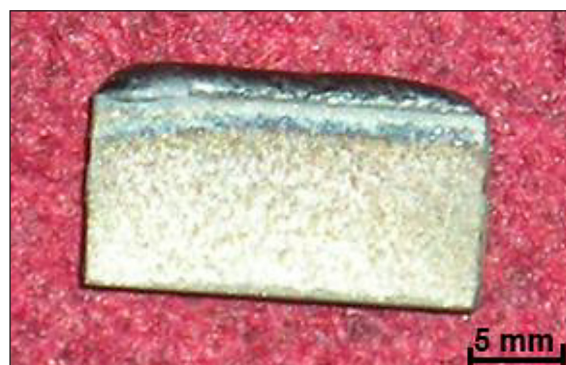
Figure 8. Appearance of the sample after laser remelting of the coating
