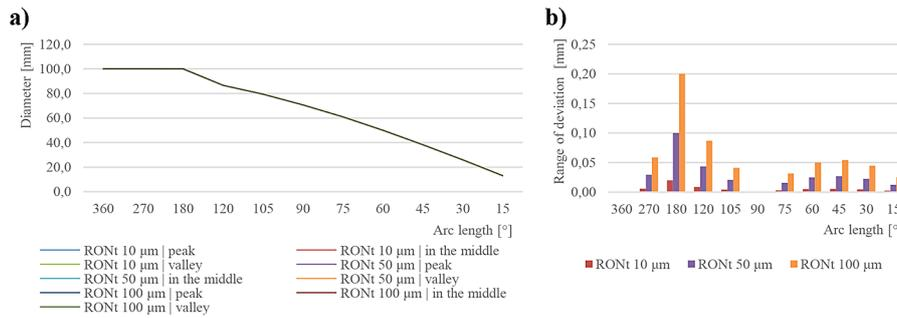
**Figure 14.** Minimum circumscribed circle (MCCI) – measurement results of a diameter of 100 mm with different deviation values: a) diameter, b) range of deviation
