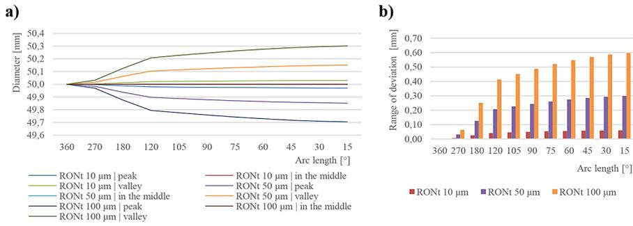
**Figure 7.** Minimum zone reference circles (MZCI) – measurement results of a diameter of 50 mm with different deviation values: a) diameter, b) range of deviation
