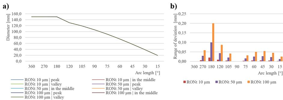
**Figure 18.** Minimum circumscribed circle (MCCI) – measurement results of a diameter of 150 mm with different deviation values: a) diameter, b) range of deviation
