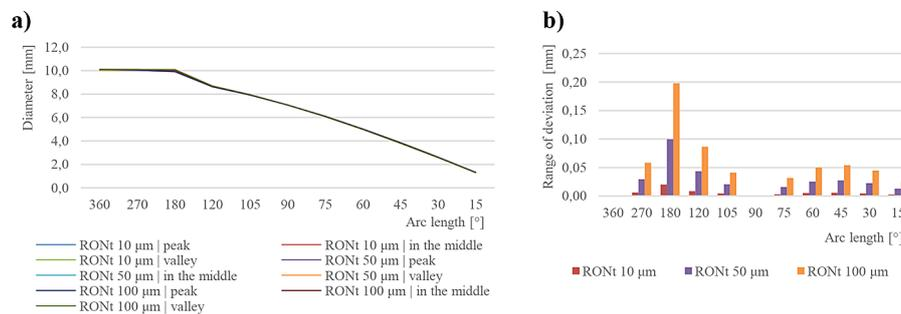
**Figure 6.** Minimum circumscribed circle (MCCI) – measurement results of a diameter of 10 mm with different deviation values: a) diameter, b) range of deviation
