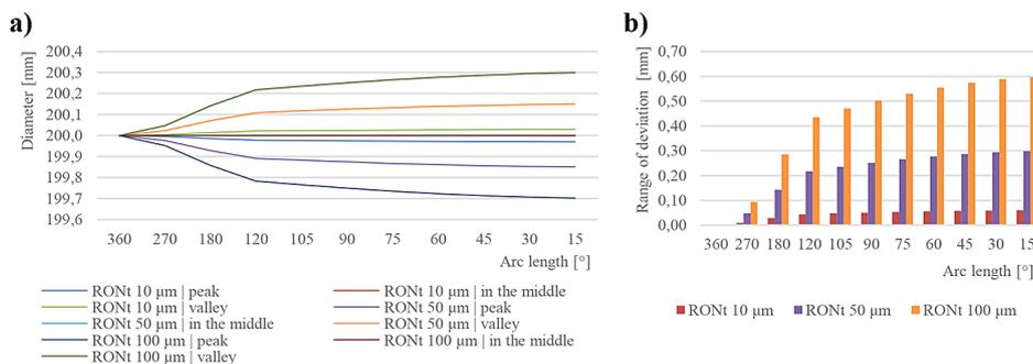
**Figure 20.** Least squares reference circle (LSCI) – measurement results of a diameter of 200 mm with different deviation values: a) diameter, b) range of deviation
