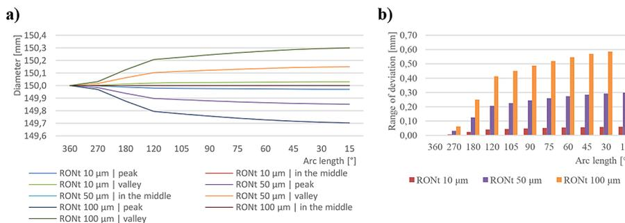
**Figure 15.** Minimum zone reference circles (MZCI) – measurement results of a diameter of 150 mm with different deviation values: a) diameter, b) range of deviation
