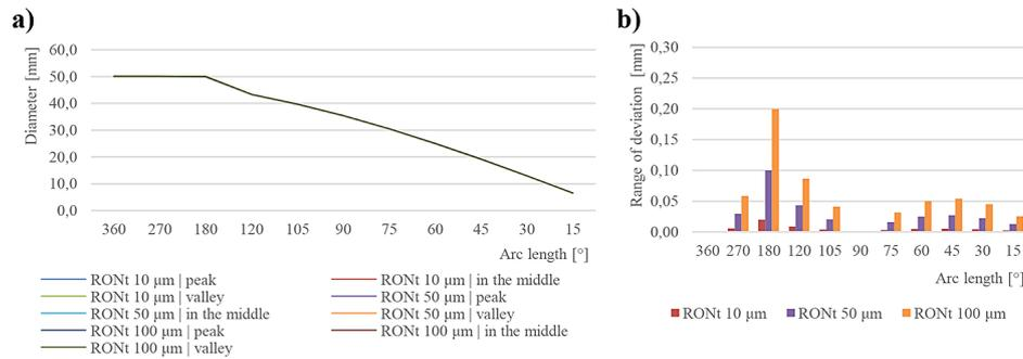
**Figure 10.** Minimum circumscribed circle (MCCI) – measurement results of a diameter of 50 mm with different deviation values: a) diameter, b) range of deviation
