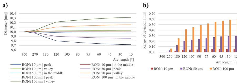
**Figure 3.** Minimum zone reference circle (MZCI) - Measurement results of a diameter of 10 mm with different deviation values: a) diameter, b) range of deviation
