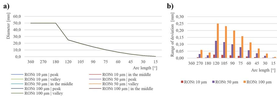
**Figure 9.** Maximum inscribed circle (MICI) – measurement results of a diameter of 50 mm with different deviation values: a) diameter, b) range of deviation
