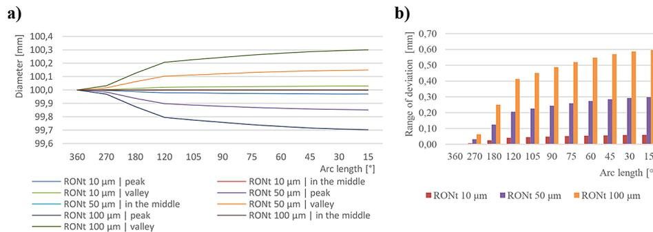
**Figure 11.** Minimum zone reference circles (MZCI) – measurement results of a diameter of 100 mm with different deviation values: a) diameter, b) range of deviation
