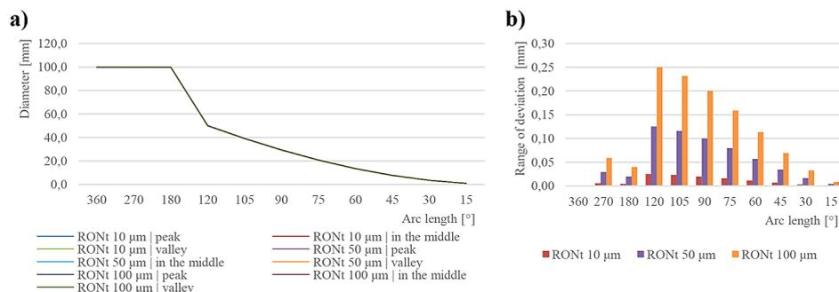
**Figure 13.** Maximum inscribed circle (MICI) – measurement results of a diameter of 100 mm with different deviation values: a) diameter, b) range of deviation
