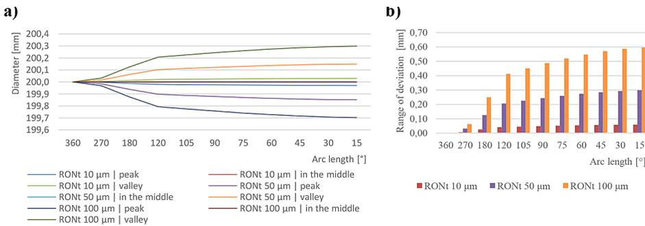
**Figure 19.** Minimum zone reference circles (MZCI) – measurement results of a diameter of 200 mm with different deviation values: a) diameter, b) range of deviation
