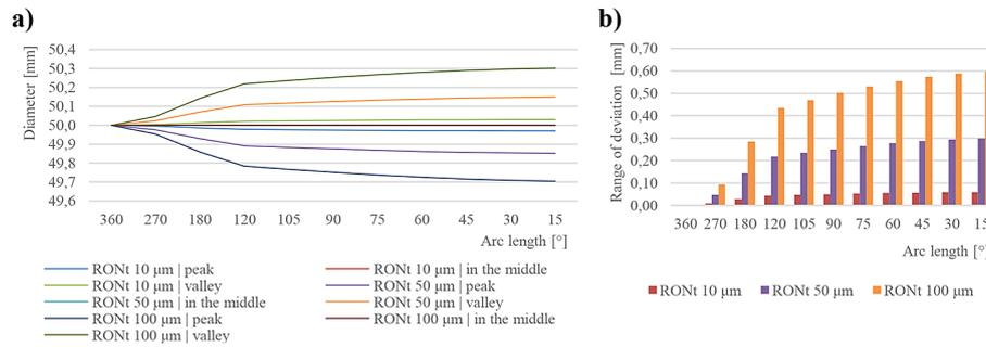
**Figure 8.** Least squares reference circle (LSCI) – measurement results of a diameter of 50 mm with different deviation values: a) diameter, b) range of deviation
