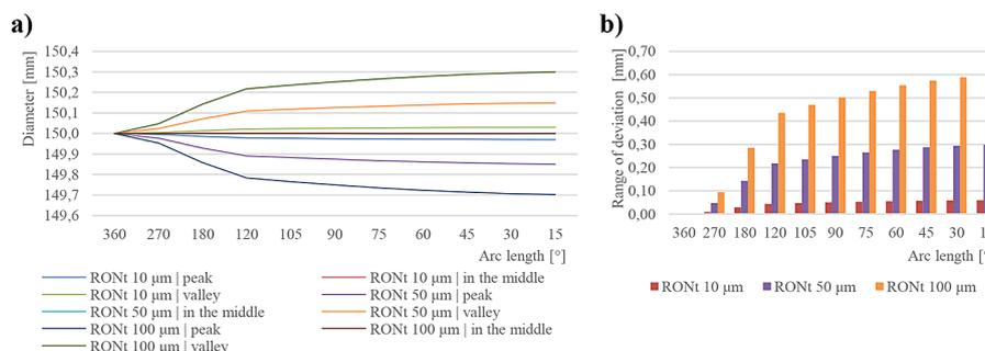
**Figure 16.** Least squares reference circle (LSCI) – measurement results of a diameter of 150 mm with different deviation values: a) diameter, b) range of deviation
