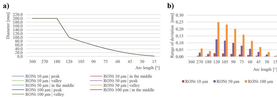
**Figure 21.** Maximum inscribed circle (MICI) – measurement results of a diameter of 200 mm with different deviation values: a) diameter, b) range of deviation
