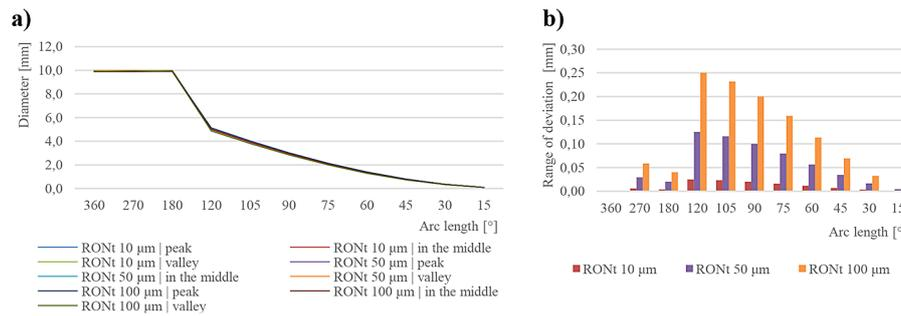
**Figure 5.** Maximum inscribed circle (MICI) – measurement results of a diameter of 10 mm with different deviation values: a) diameter, b) range of deviation
