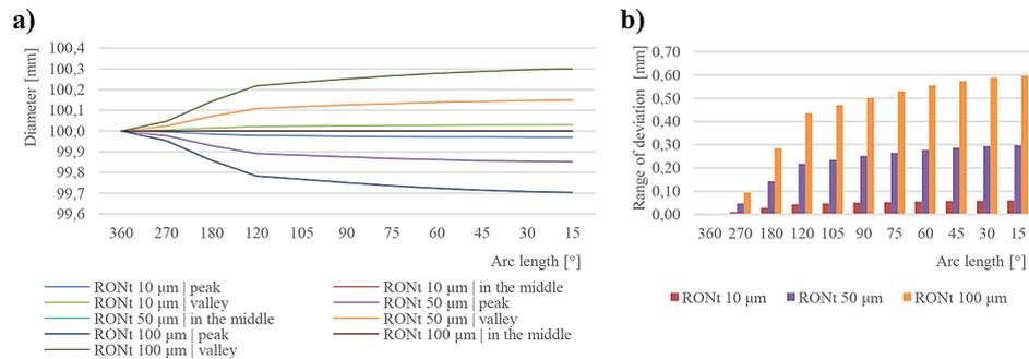
**Figure 12.** Least squares reference circle (LSCI) – measurement results of a diameter of 100 mm with different deviation values: a) diameter, b) range of deviation
