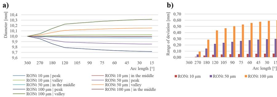
**Figure 4.** Least squares reference circle (LSCI) - Measurement results of a diameter of 10 mm with different deviation values: a) diameter, b) range of deviation
