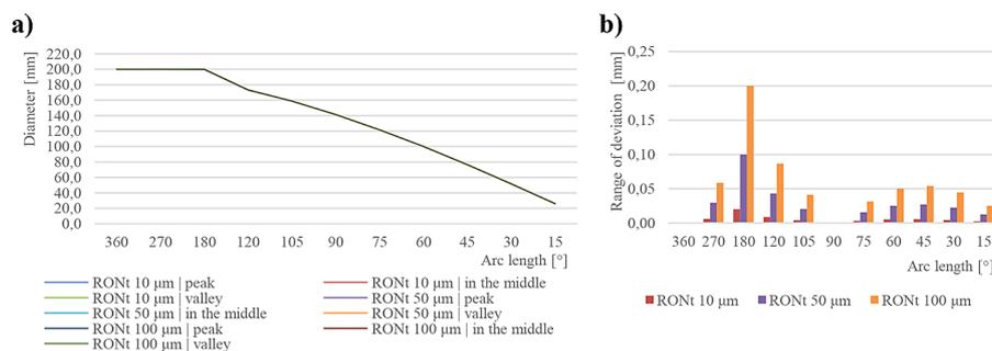
**Figure 22.** Minimum circumscribed circle (MCCI) – measurement results of a diameter of 200 mm with different deviation values: a) diameter, b) range of deviation
