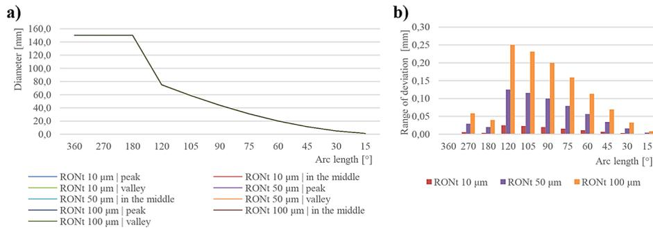
**Figure 17.** Maximum inscribed circle (MICI) – measurement results of a diameter of 150 mm with different deviation values: a) diameter, b) range of deviation
