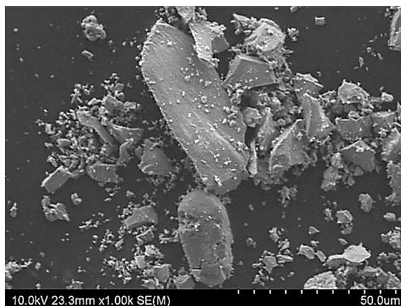
Figure 4. SEM microstructure of  $\text{ZrSiO}_4$
