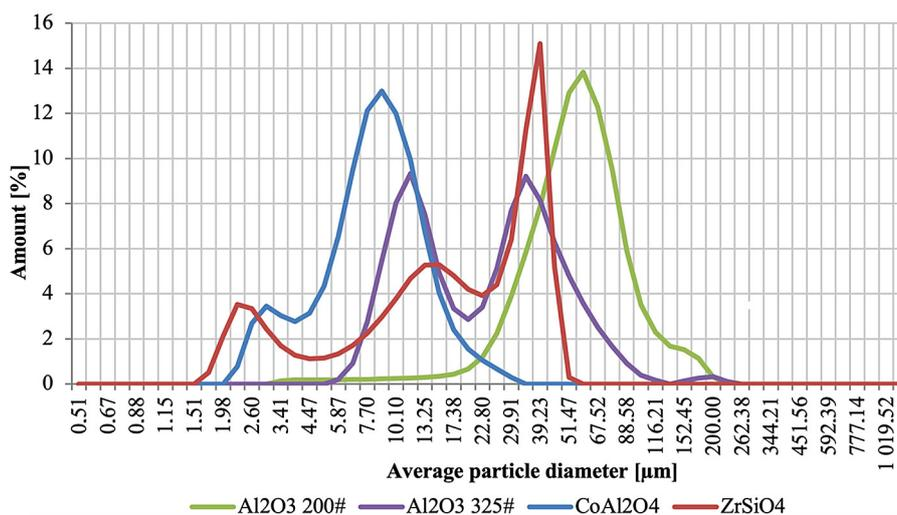
Figure 5. Distribution of the average particle diameter of powders used for prime coats – Al<sub>2</sub>O<sub>3</sub> 200#, Al<sub>2</sub>O<sub>3</sub> 325#, CoAl<sub>2</sub>O<sub>4</sub>, ZrSiO<sub>4</sub>
