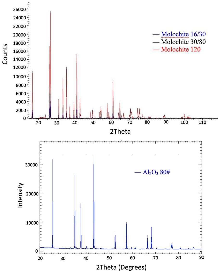
**Figure 13.** Diffraction diagrams of Molochite 16/30, Molochite 30/80, Molochite 120 and  $\text{Al}_2\text{O}_3$  80#
