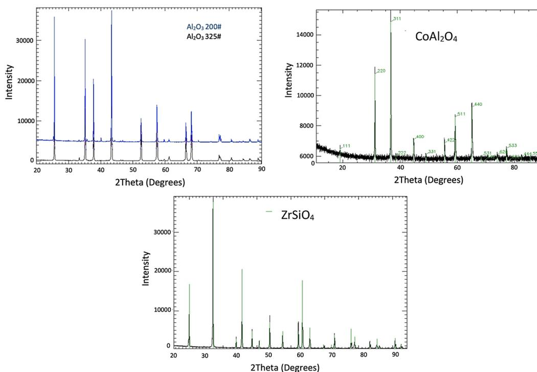
**Figure 7.** Diffraction diagrams of the powders
