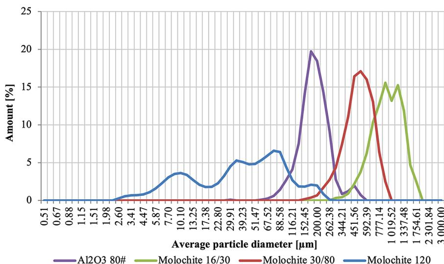
Figure 12. Distribution of the average particle diameter of powders used for backup layers – Al<sub>2</sub>O<sub>3</sub> 80#, Molochite 16/30, Molochite 30/80, Molochite 120
