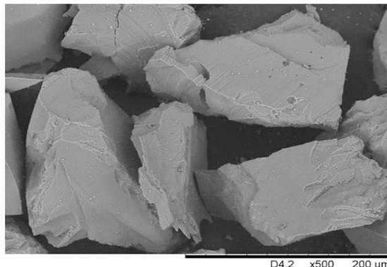
Figure 11. SEM microstructure of Al<sub>2</sub>O<sub>3</sub> 80#
