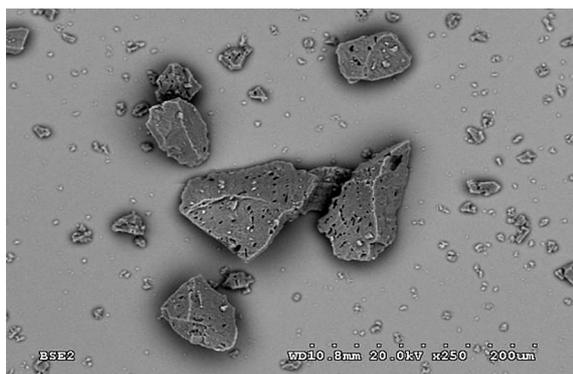
Figure 10. SEM microstructure of Molochite 120
