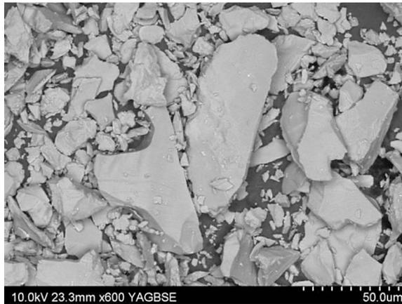
Figure 2. SEM microstructure of  $\text{Al}_2\text{O}_3$  325#
