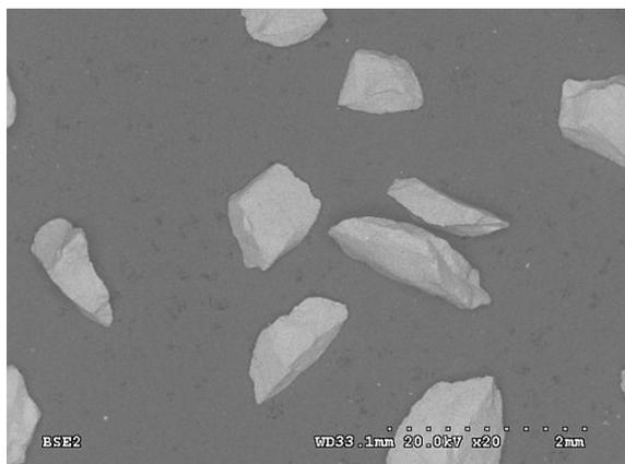
**Figure 8.** SEM microstructure of Molochite 16/30
