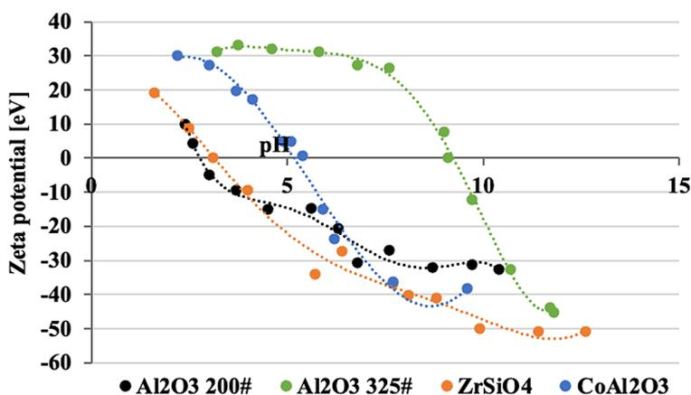
Figure 6. Distribution of Zeta potential of ceramic powders – Al<sub>2</sub>O<sub>3</sub> 200#, Al<sub>2</sub>O<sub>3</sub> 325#, ZrSiO<sub>4</sub>, CoAl<sub>2</sub>O<sub>4</sub>
