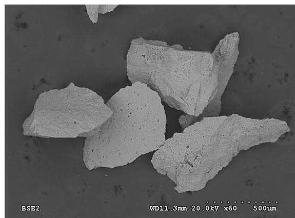
**Figure 9.** SEM microstructure of Molochite 30/80
