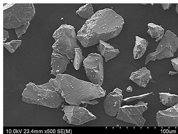
Figure 1. SEM microstructure of  $\text{Al}_2\text{O}_3$  200#
