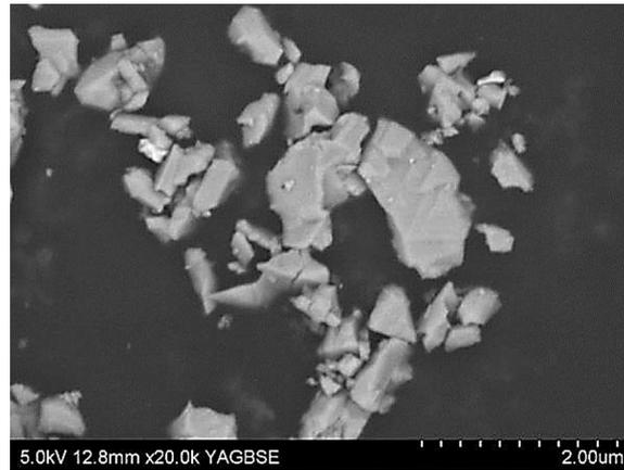
Figure 3. SEM microstructure of  $\text{CoAl}_2\text{O}_4$
