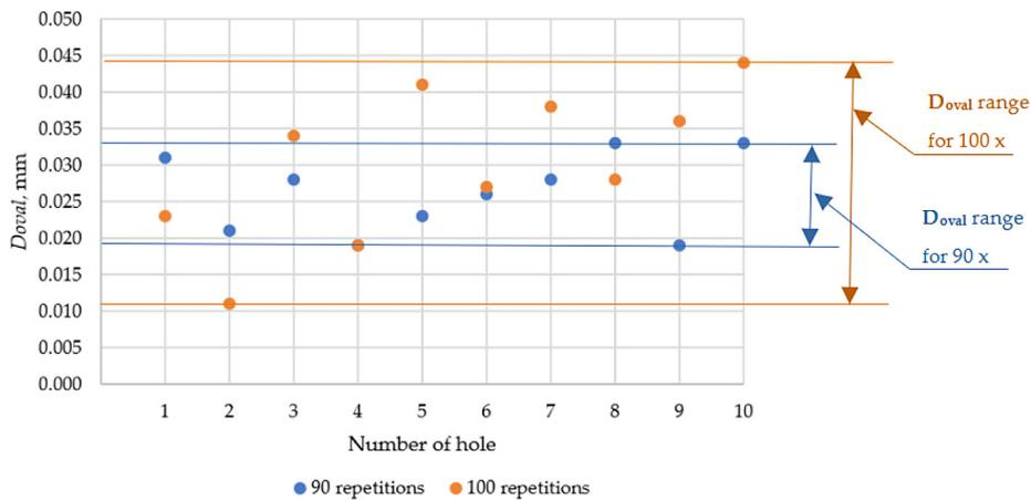
Figure 5. Comparison of the degree of deviation of the holes from the actual outline with a diameter of 1 mm
