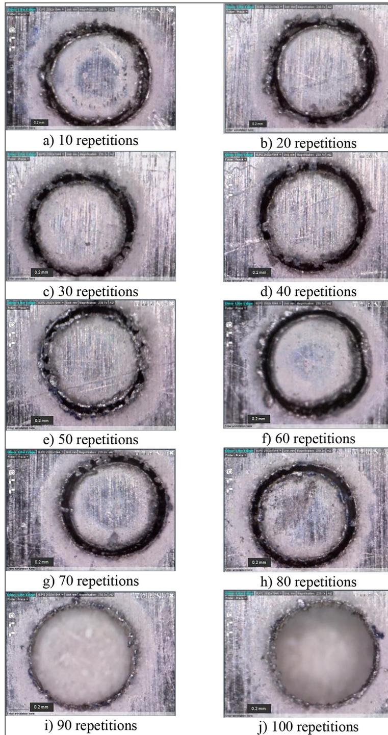
**Figure 3.** Cutting the 1 mm diameter hole by repeating the number of beam passes: (a) 10×, (b) 20×, (c) 30×, (d) 40×, (e) 50×, (f) 60×, (g) 70×, (h) 80×, (i) 90×, (j) 100× (mag. app. 200×)
