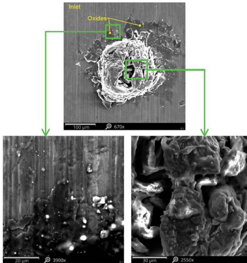
Figure 13. SEM images of the 0.1 mm diameter hole
