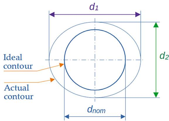
**Figure 4.** The adopted rules for measuring the diameter of the hole:  $d_{nom}$  – nominal value of the hole diameter,  $d_1$  and  $d_2$  – diameter values measured perpendicular to each other
