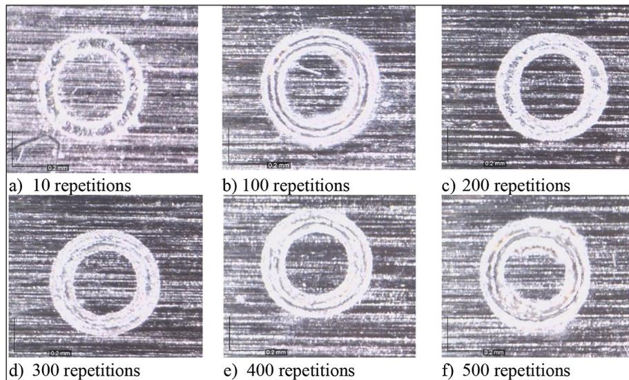
**Figure 8.** Results of hole cutting tests according to the selected variant: a) 10 repetitions, b) 100 repetitions, c) 200 repetitions, d) 300 repetitions, e) 400 repetitions, f) 500 repetitions (mag. app. 200×)
