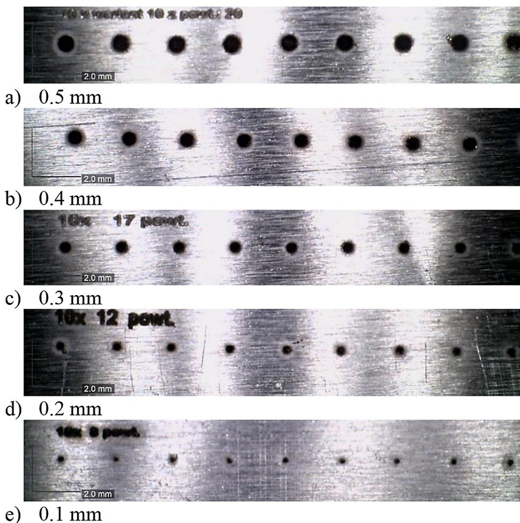
Figure 11. Micro holes made for measuring purposes (mag. app. 20×)
