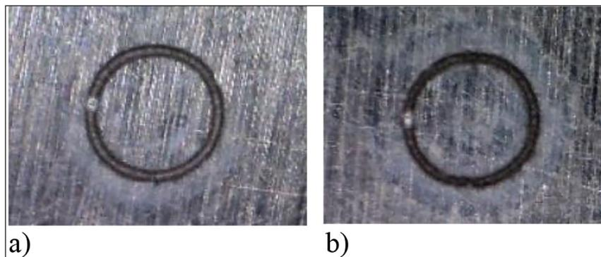
Figure 2. Comparison of holes made with the same pulse frequency and power but different speeds, (a) 100 mm/s, (b) 50 mm/s
