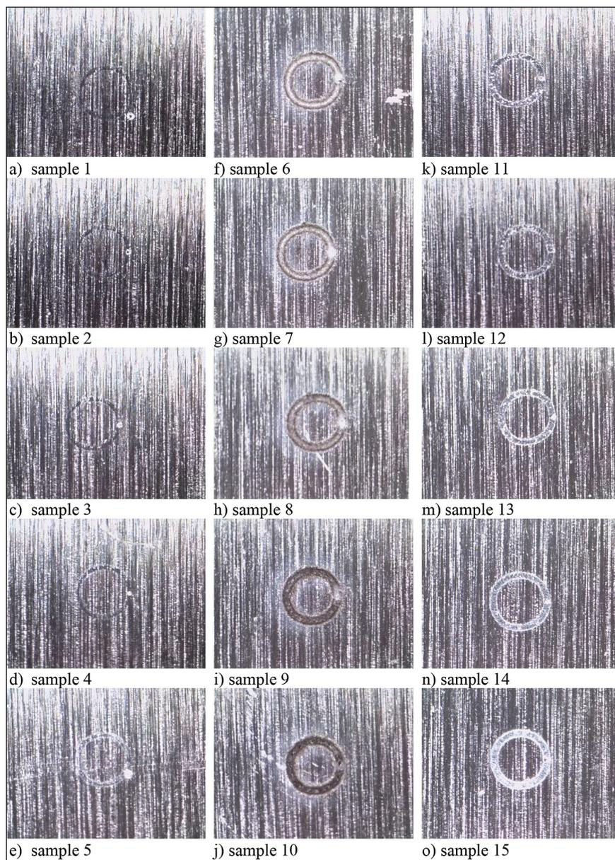
**Figure 7.** Results of the trial machining of a 0.5 mm hole with one pass of the laser beam: (a–o) subsequent variants according to Table 4 (mag. app. 200×)
