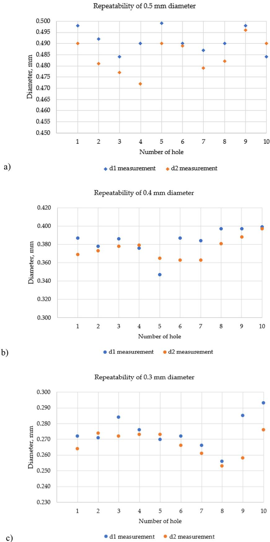
**Figure 14.** Hole sizes and their repeatability for diameters: a) 0.5 mm, b) 0.4 mm, c) 0.3 mm, d) 0.2 mm, e) 0.1 mm
