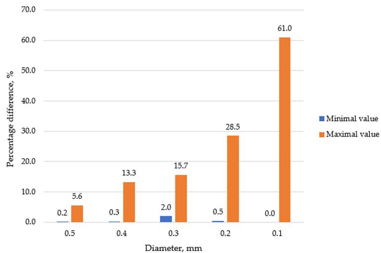
Figure 15. Percentage loss of hole accuracy
