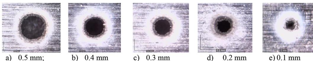
Figure 10. Micro holes obtained with a fixed number of repetitions (mag. app. 200×)
