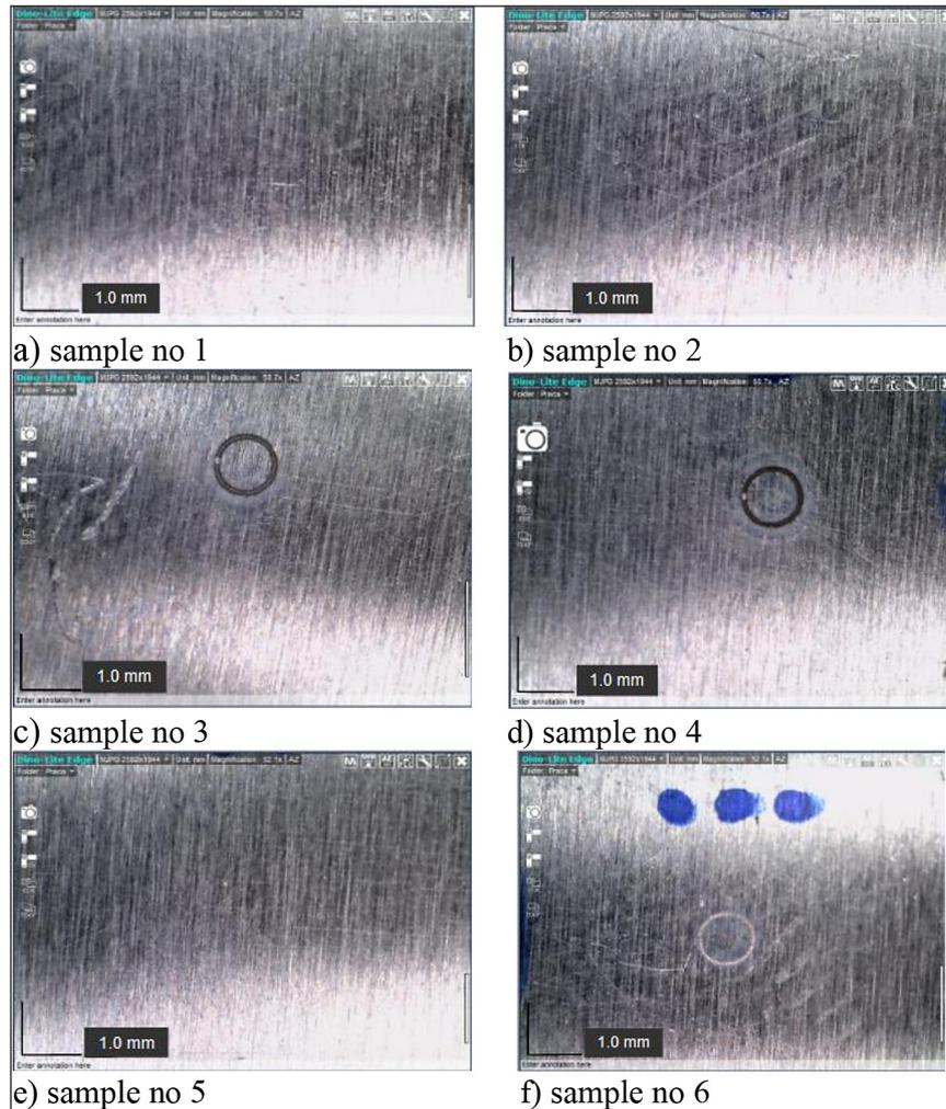
Figure 1. Results of trial cutting of 1 mm diameter holes: (a÷f) samples in the preliminary test (mag. app. 50×)
