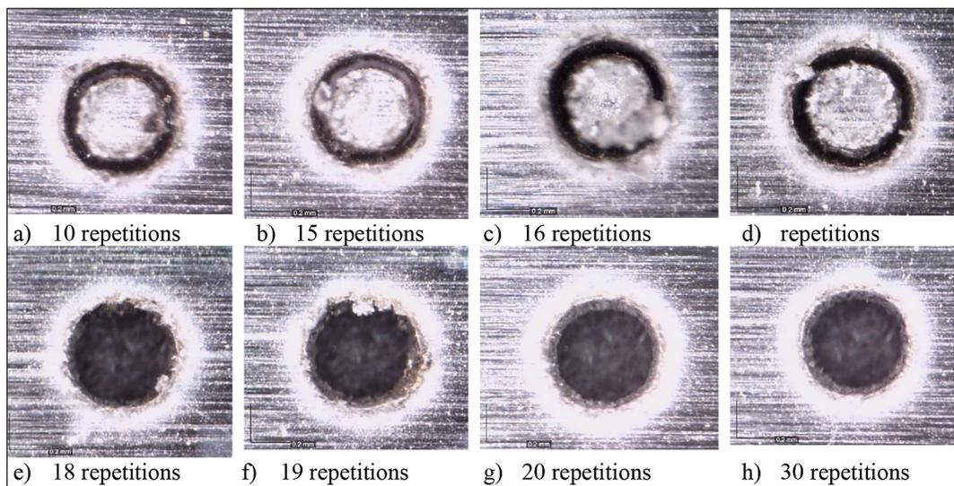
**Figure 9.** Test hole cutting results with the selected number of passes: a) 10, b) 15, c) 16, d) 17, e) 18, f) 19, g) 20, h) 30 (mag. app. 200×)
