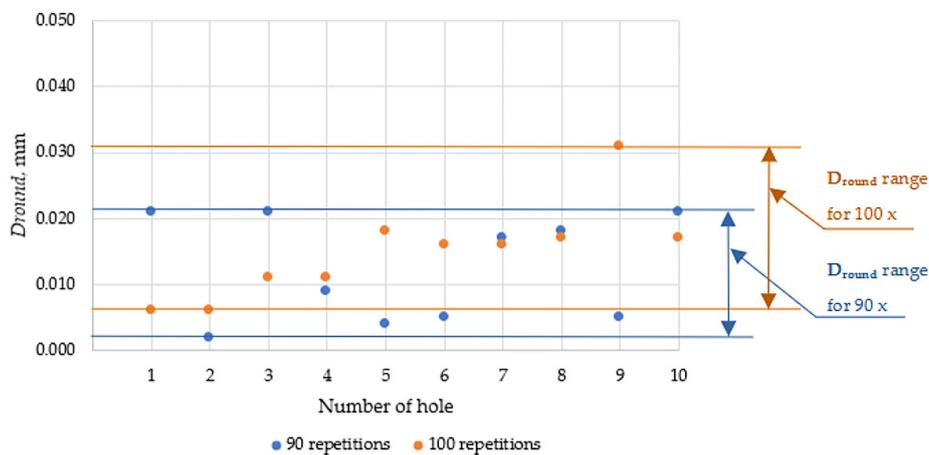
Figure 6. Comparison of the roundness of 1 mm diameter holes
