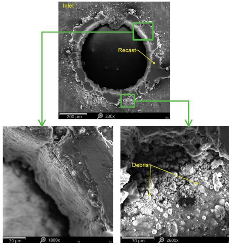
Figure 12. SEM images of the 0.5 mm diameter hole
