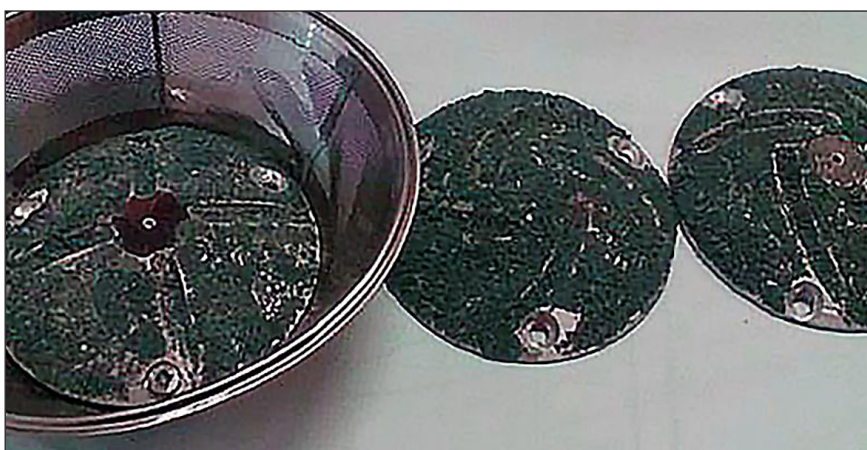
Figure 7. Abrasive discs with curved grooves [60]
