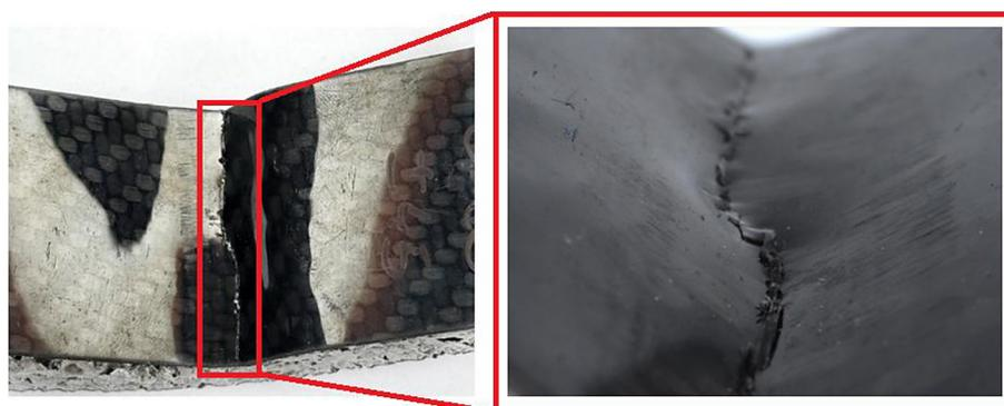
Figure 15. Fracture line for CFPR cladding based on C2 specimen (zoom x20)
