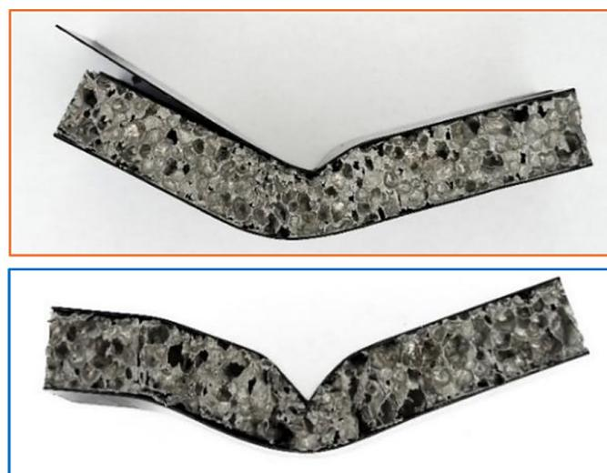
Figure 10. Frontal view of tested C2 specimen
