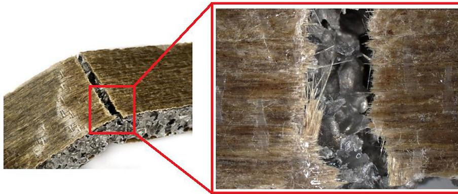
**Figure 16.** Total damage of the lower flax cladding for the F1-S1 specimen (zoom x20)
