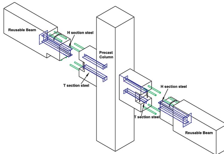
Figure 17. Beam-to-column connections [7]
