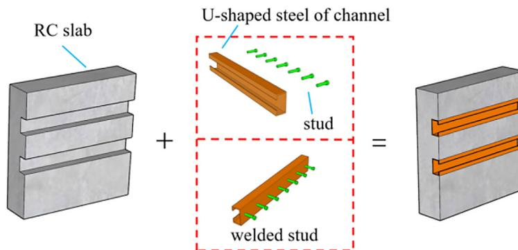
Figure 14. Friction-based connector [32]
