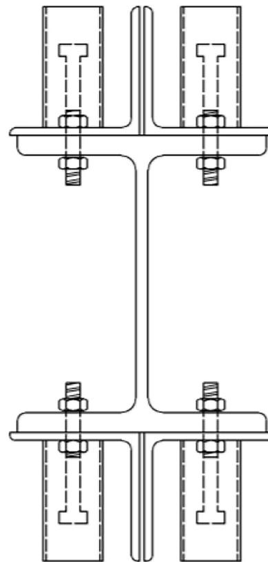
**Figure 9.** Injection bolt [20]
