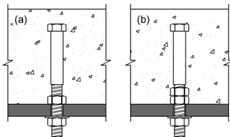
Figure 4. Single (a) and double nut configurations (b) [8]
