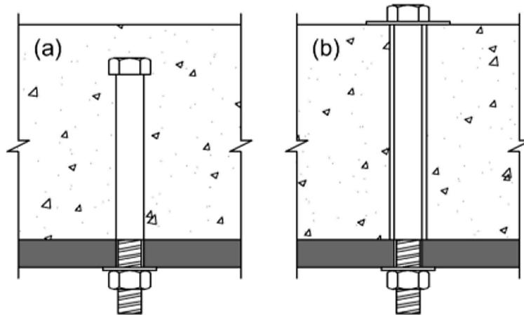
Figure 1. No embedded nut (a), friction grip bolt (b) [8]
