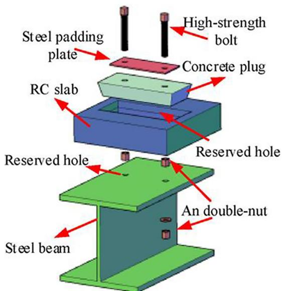
Figure 15. Steel-yielding connector [23]
