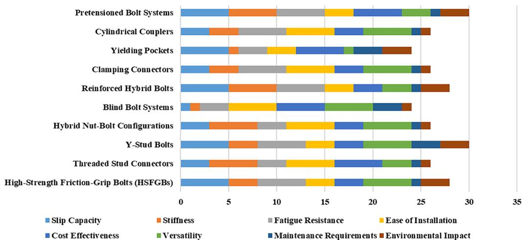
Figure 21. Performance characteristics of connectors
