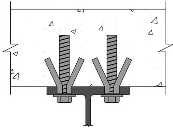
Figure 5. Blind bolt concealed connections [16]
