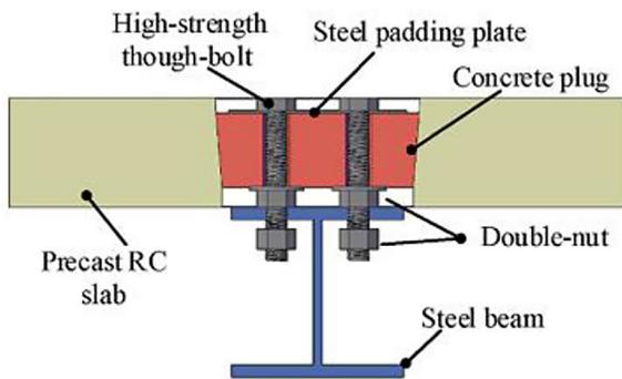
Figure 13. Locking nut high-performance connection [19]
