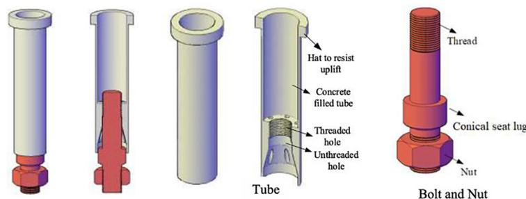
Figure 7. Locking nut mechanisms [10]
