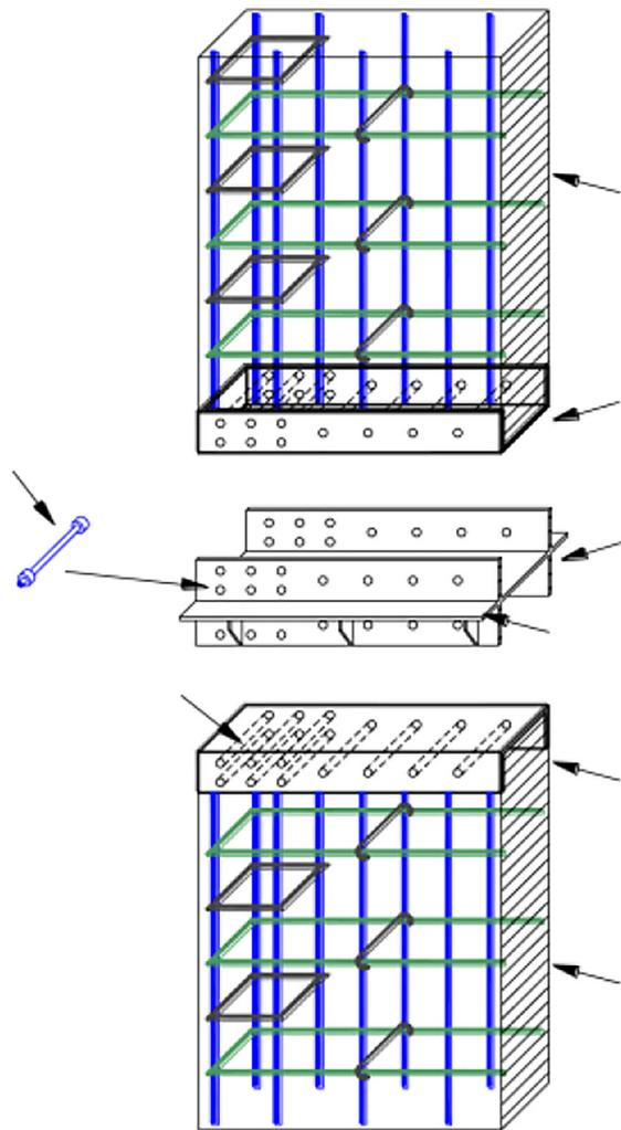
Figure 20. Wall and foundation joint techniques [42]
