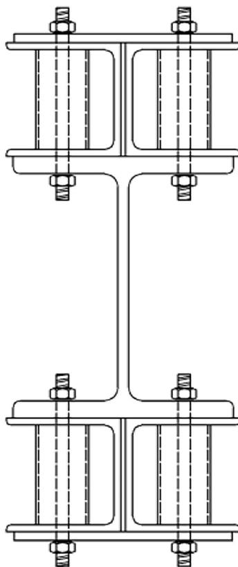
Figure 11. Clamping couplers [20]
