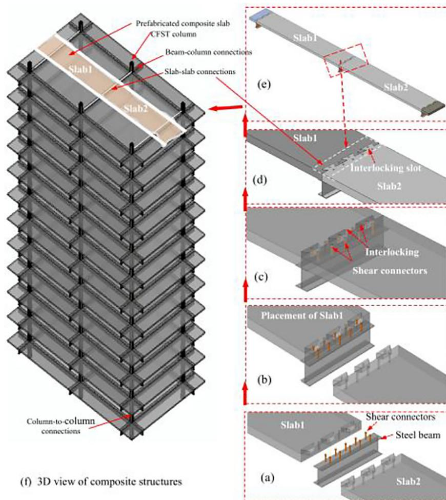
Figure 19. Slab and beam joint techniques [14]
