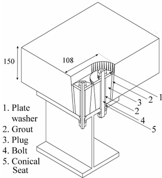
Figure 12. Locking-bolt system [22]
