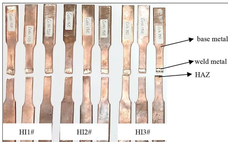
Figure 5. Tensile fracture on the welded specimen
