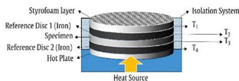
Figure 2. Schematic of thermal conductivity measurement (23)
