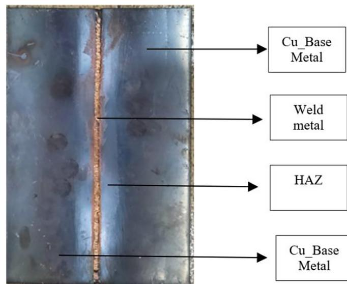
Figure 3. Welded joint of copper material
