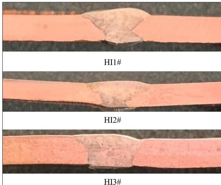
Figure 4. Macro view of three heat input variations
