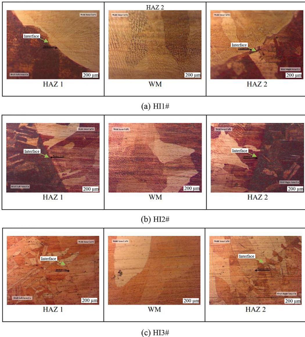
**Figure 10.** Microstructure test results for different heat input
