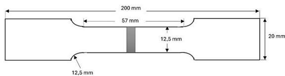
Figure 1. Tensile test specimen (22)
