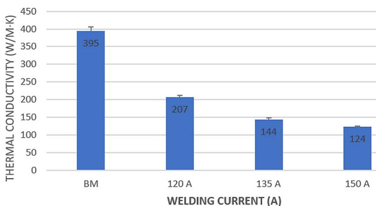
Figure 9. Thermal conductivity values of welded copper joints and standard deviation
