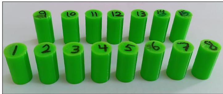
Figure 3. 3D printed PETG samples for compressive strength tests
