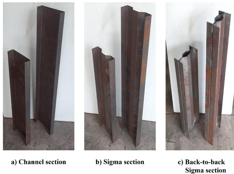
Figure 1. Fabricated specimens
