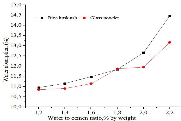
Figure 9. Water absorption of concrete wall panel specimens with different water-to-binder weight ratios
