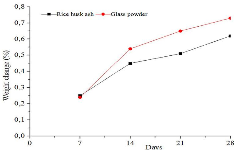
Figure 11. Weight change of concrete wall panels specimen during treatment with hydrochloric acid
