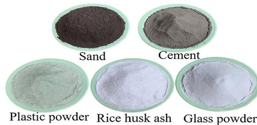
**Figure 1.** Materials for precast concrete wall panels preparation
