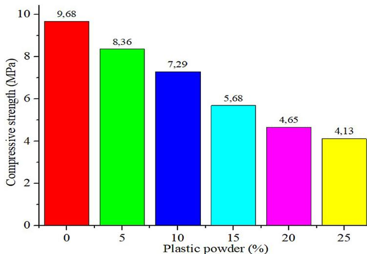
Figure 4. Compressive strength of concrete wall panels as a function of partial replacement of sand with plastic powder
