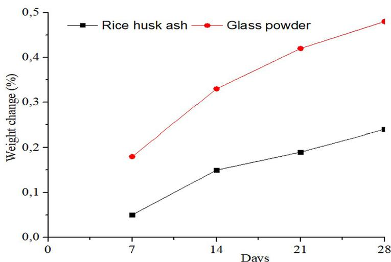
Figure 10. Weight change of concrete wall panels specimen during treatment with sulfate
