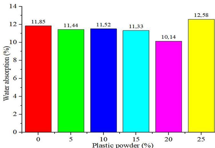
**Figure 5.** Water absorption of concrete wall panels as a function of partial replacement of sand with plastic powder
