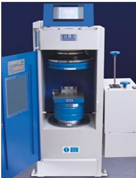
Figure 2. ADR touch compressive testing machine
