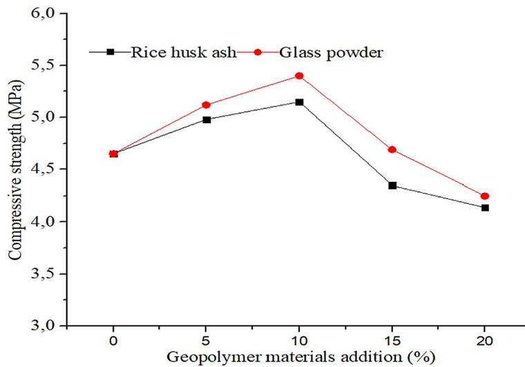
Figure 6. Compressive strength of concrete wall panels as a function of partial replacement of cement with silica-rich recycled materials
