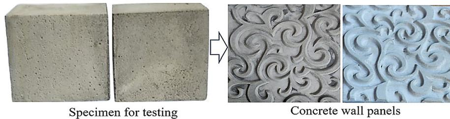
Figure 3. Physical appearance of concrete containing plastic waste and recycled materials
