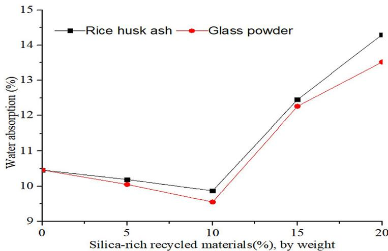
Figure 7. Water absorption of concrete wall panels composed with 20% plastic powder and different addition of silica-rich recycled materials
