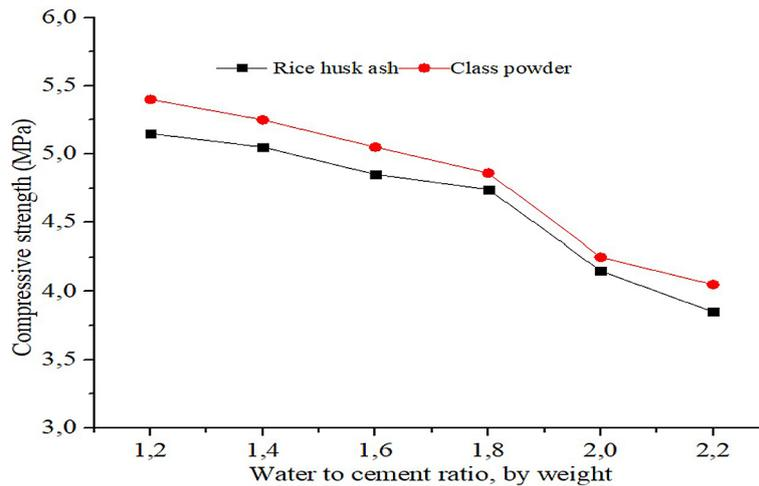
Figure 8. Compressive strength of concrete wall panels specimen with different water-to-binder weight ratios
