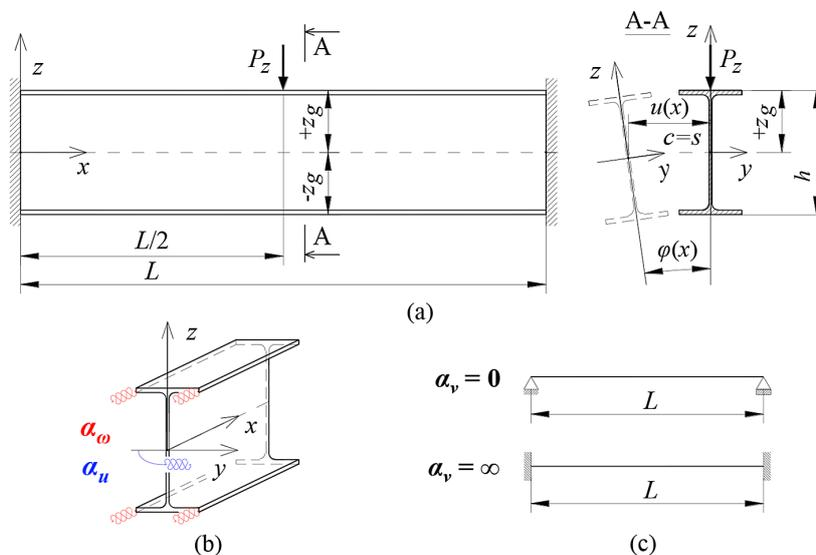
**Figure 1.** (a) Static scheme of a beam loaded with concentrated force, (b) Elastic stiffnesses at the support node, (c) Conditions for fixing the beam in the bending plane
