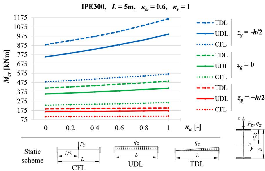
**Figure 5.** Trends in  $M_{cr}(\kappa_u)$  variation according to *LTBeamN* software for bilaterally fixed ( $\kappa_v = 1$ ) IPE300 beam ( $L = 5$  m)
