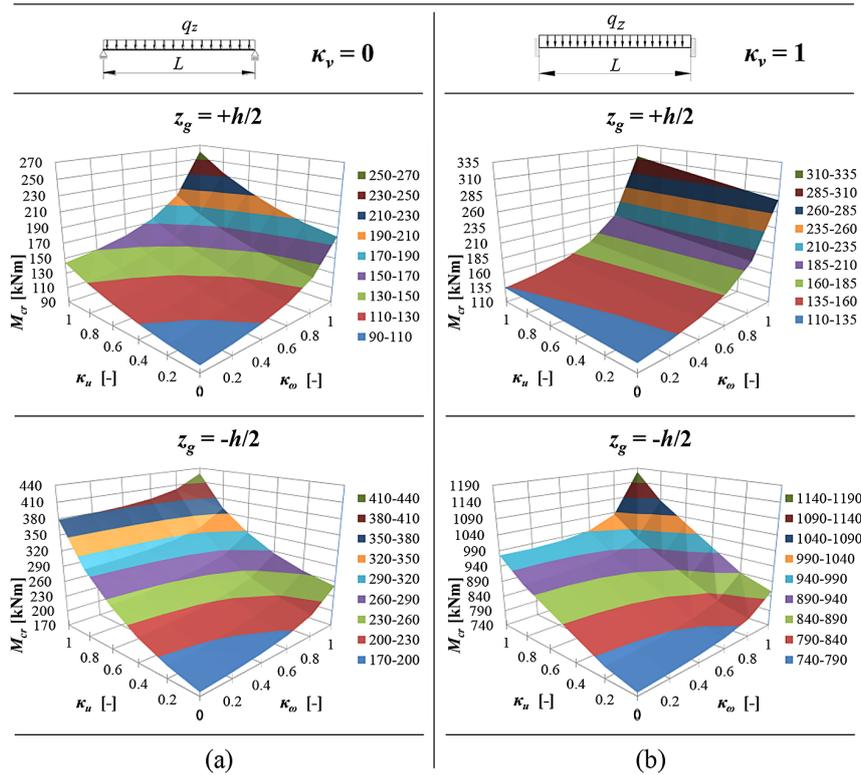
Figure 6. Trends in  $M_{cr}(\kappa_{\omega}, \kappa_u)$  variation according to formula (5) for a uniformly loaded beam: (a) simply supported beam ( $\kappa_v = 0$ ), (b) bilaterally fixed beam ( $\kappa_v = 1$ )
