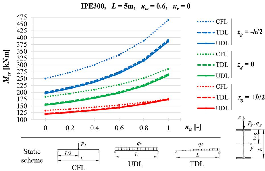
**Figure 2.** Trends in  $M_{cr}(\kappa_u)$  variation according to *LTBeamN* software for simply supported ( $\kappa_v = 0$ ) IPE300 beam ( $L = 5$  m)
