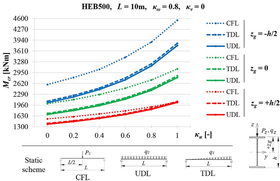
Figure 4. Trends in  $M_{cr}(\kappa_u)$  variation according to *LTBeamN* software for simply supported ( $\kappa_v = 0$ ) HEB500 beam ( $L = 10$  m)
