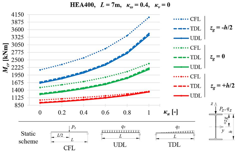
Figure 3. Trends in  $M_{cr}(\kappa_u)$  variation according to *LTBeamN* software for simply supported ( $\kappa_v = 0$ ) HEA400 beam ( $L = 7$  m)
