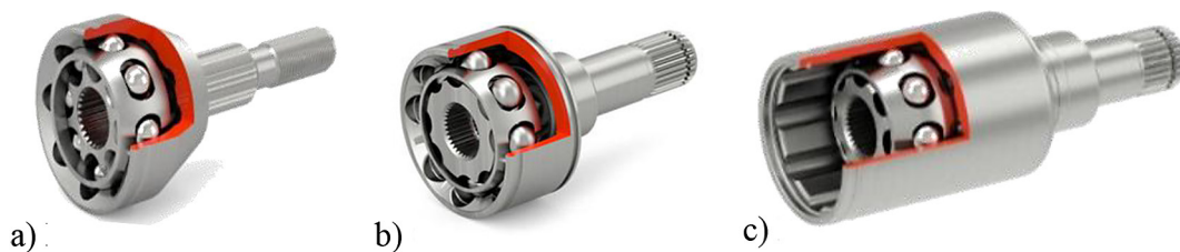
Figure 2. Main types of constant-velocity joints (a) Rzeppa, (b) cross groove, (c) double offset
