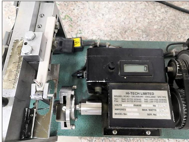
Figure 9. Alternative bending fatigue machine
