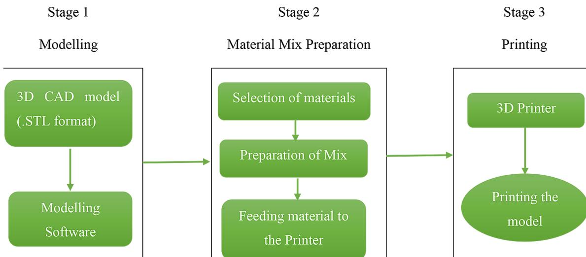
Figure 4. Stages of 3D printing
