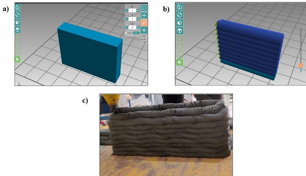
**Figure 5.** Modelling and printing a) 3D modelling (.stl file) b) 3D slicing the model c) 3D concrete printing
