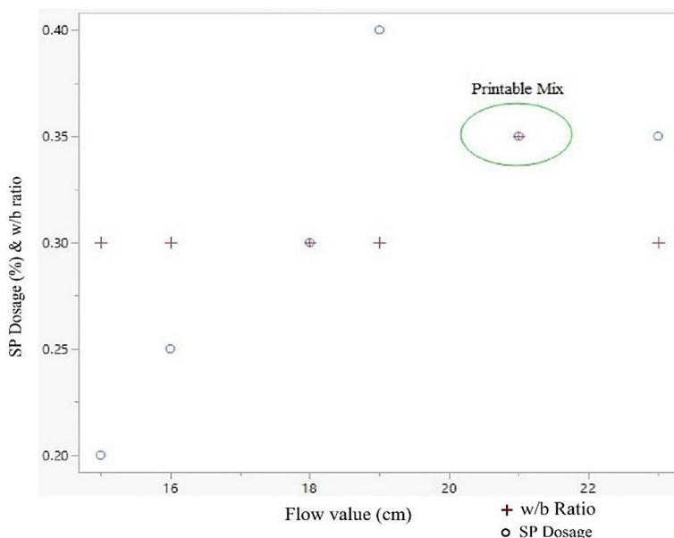
Figure 11. Printable mix with flow value, w/b ratio and SP dosage(%)
