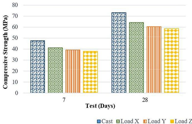
**Figure 12.** Compressive strength of the cast and printed specimens (Loaded along X, Y, and Z directions) at 7 and 28 days
