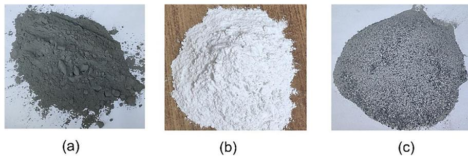
**Figure 1.** Raw materials used in 3DCP mix (a) cement; (b) marble powder; (c) M-sand
