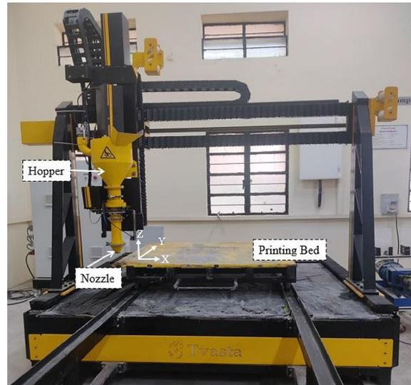
Figure 3. 3D printer
