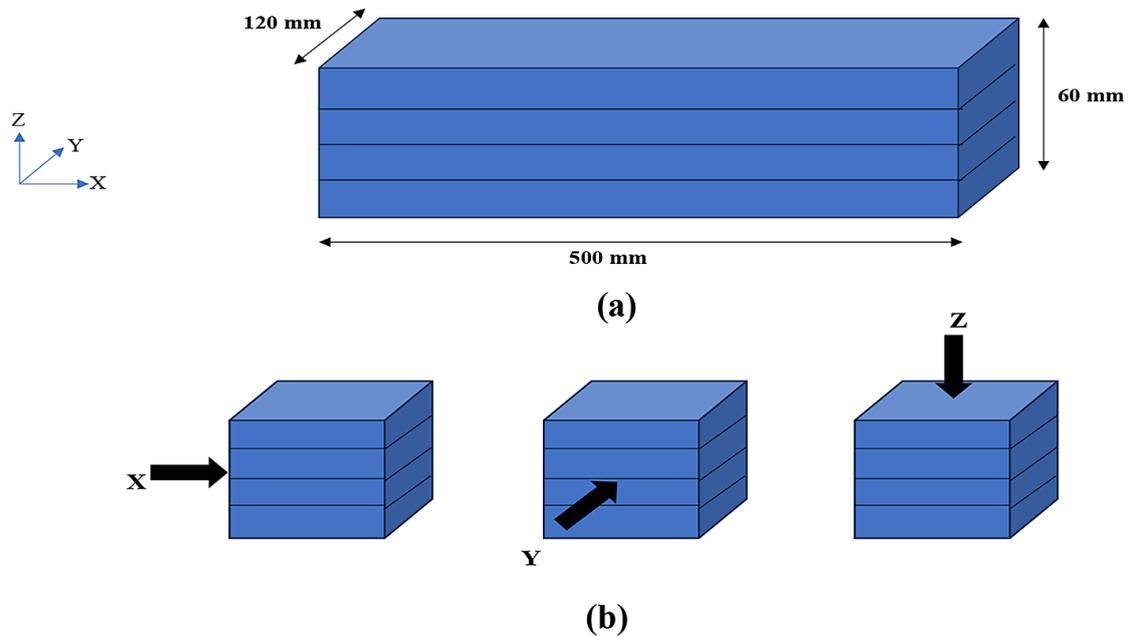
Figure 6. (a) Printed specimen (b) X, Y, and Z loading direction in the test specimens of 50 mm cube
