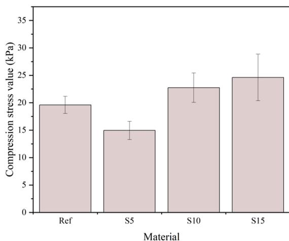
**Figure 10.** CV40 value of the obtained foams
