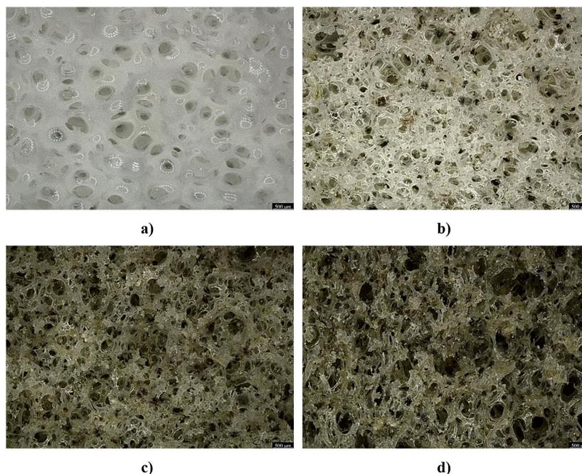
Figure 7. Micrographs of the obtained foams: Ref (a), S5 (b), S10 (c) and S15 (d)
