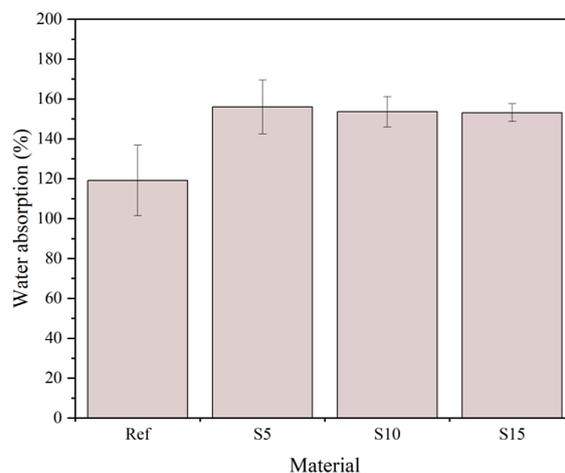
Figure 9. Water absorption of the obtained foams
