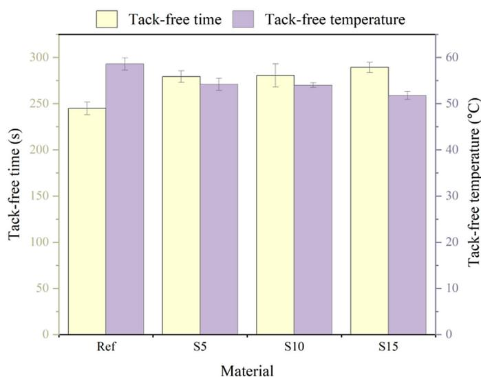
Figure 5. Tack-free time and corresponding temperature recorded for the obtained foams
