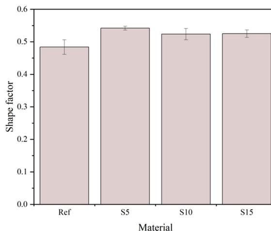
Figure 6. Variation in shape factor based on the filler content
