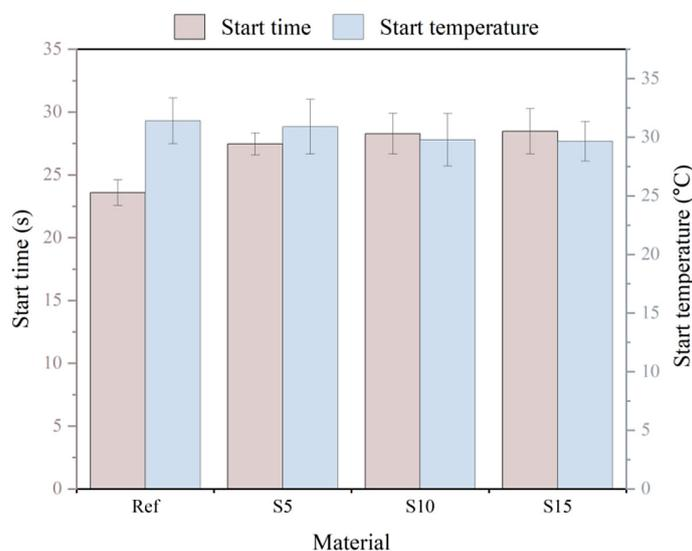
Figure 3. Start time and corresponding temperature recorded for the obtained foams
