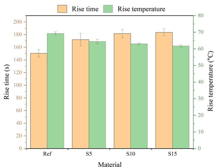
Figure 4. Rise time and corresponding temperature recorded for the obtained foams
