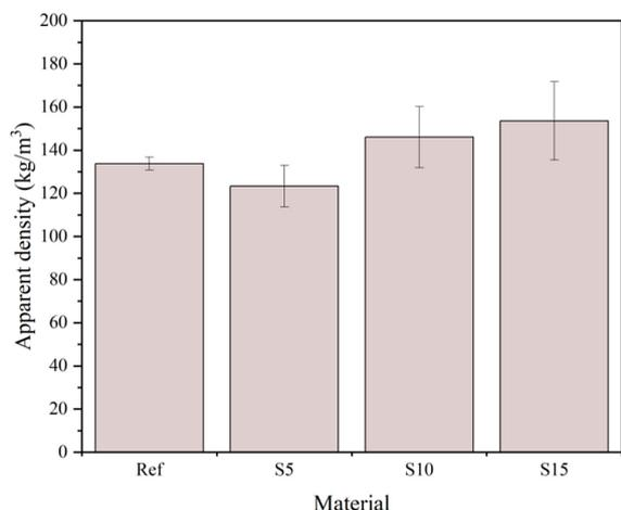
Figure 8. Apparent density of the obtained foams
