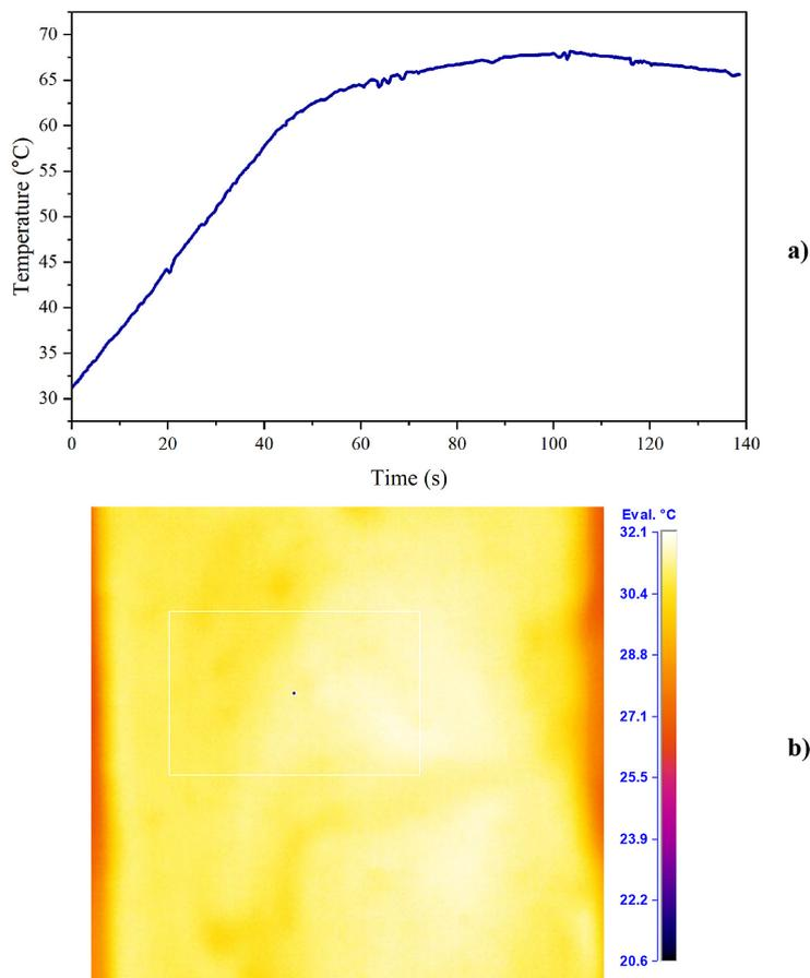
**Figure 2.** Temperature–time profile of the reference sample foaming process (a) and thermal image at the start of the process (b)
