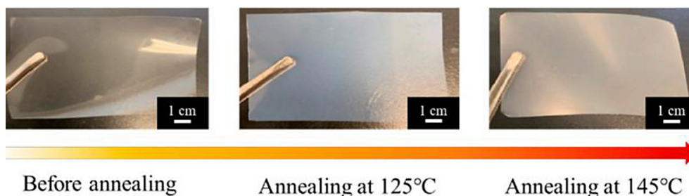
Figure 11. The effect of temperature annealing process on the appearance of piezoelectric film [76]
