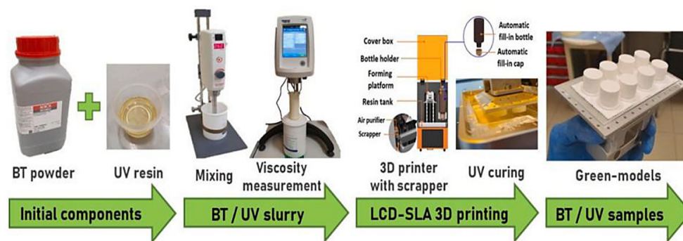
Figure 21. LCD-SLA 3D printing of BT/UV samples [90]
