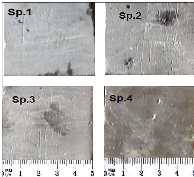
Figure 5. Specimens of thermal conductivity test
