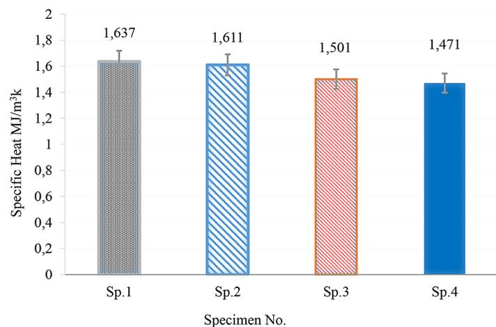
Figure 10. Specific heat coefficient for all sample with the different ratio rock wool
