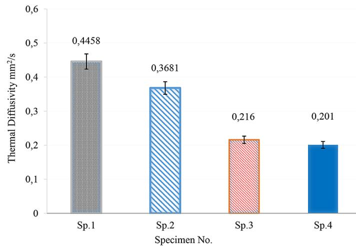
Figure 9. Thermal diffusivity coefficient for all sample with the different ratio rock wool
