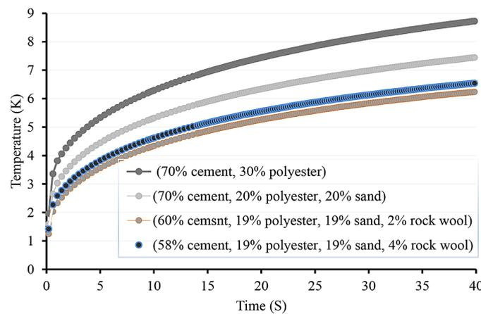
**Figure 7.** Temperature response of concrete mixtures with varying rock wool content over time
