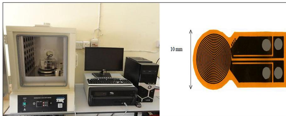
Figure 4. Device for measuring thermal properties and configuration of hot disk sensor
