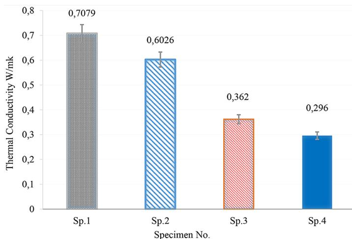
**Figure 8.** Thermal conductivity for all sample with the different ratio rock wool
