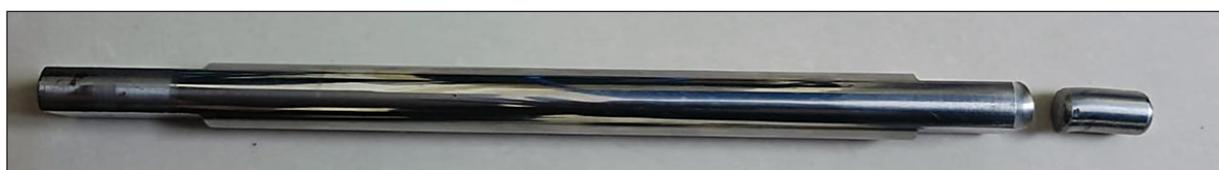
**Figure 1.** Broken butterfly valve shaft during operation
