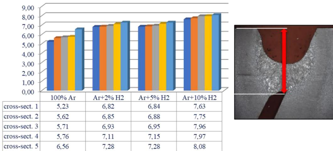
Figure 7. The depth of material melting measured from the sheet surface to the bottom of the weld [mm]
