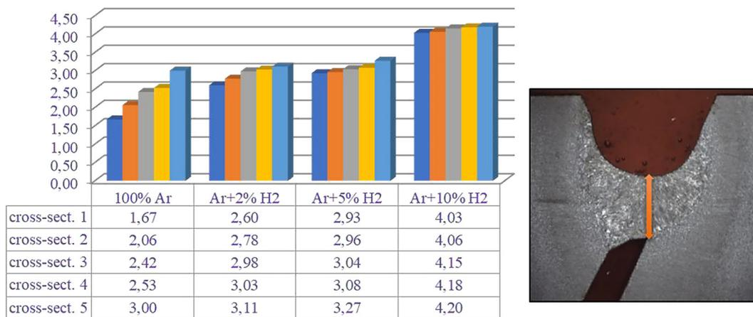
Figure 8. Thickness of the weld calculated from the face surface to the weld root [mm]
