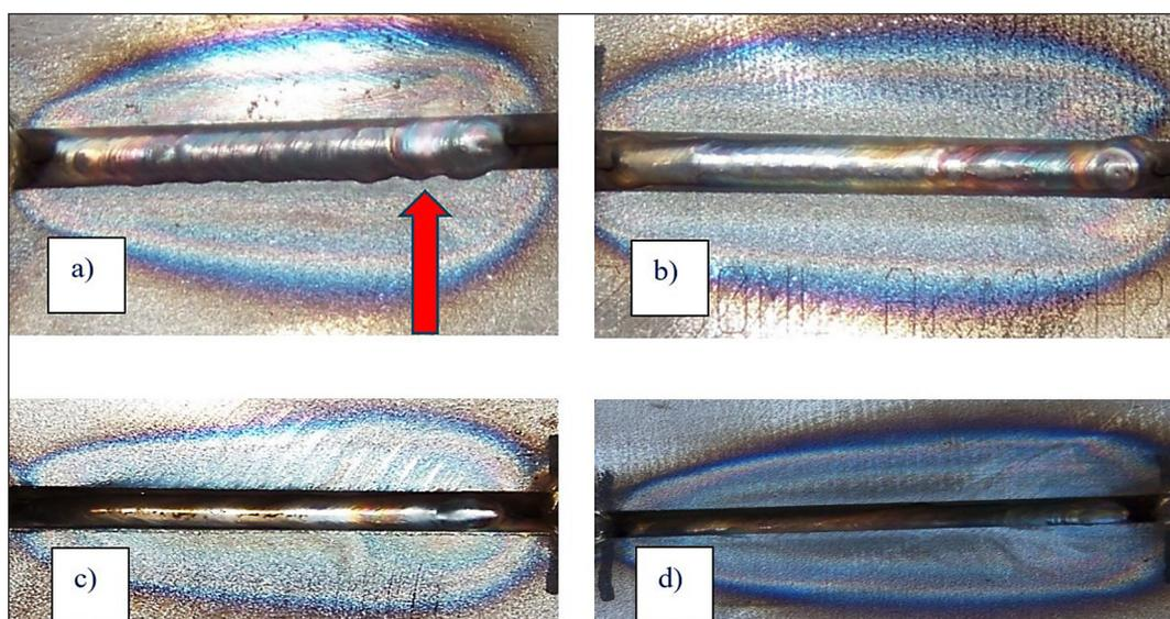
**Figure 3.** Steel plates for Tekken test, (a) S700E, gas shield 100% Ar, (b) S500ML, gas shield Ar + 2% H<sub>2</sub>, (c) S700MC, gas shield Ar + 5% H<sub>2</sub>, (d) S500ML, gas shield Ar + 10% H<sub>2</sub>
