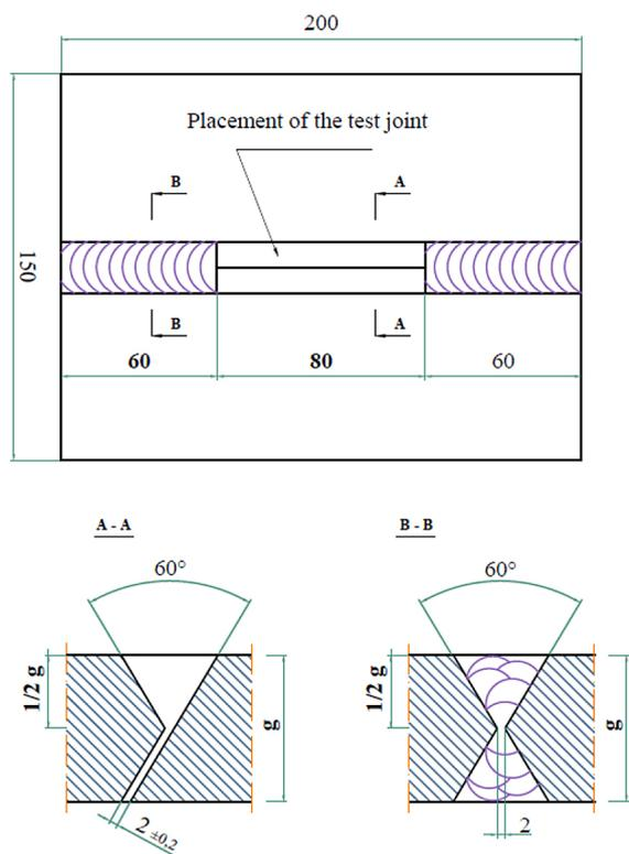
**Figure 2.** TEKKEN specimen (PN-EN ISO 17642-2:2005)
