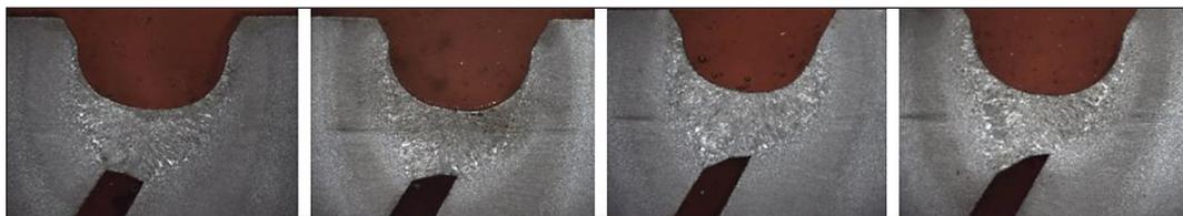
**Figure 4.** S500ML, Ar shield + 2%H<sub>2</sub>
