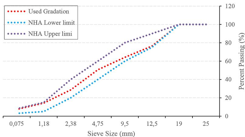
Figure 7. Blend gradation-3 for 6% filler
