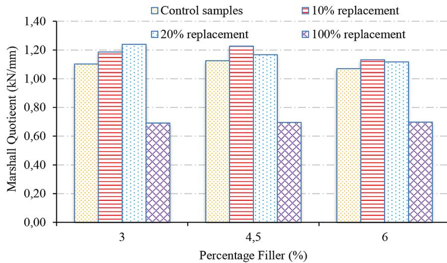
Figure 10. Marshall quotient vs filler content for different replacements
