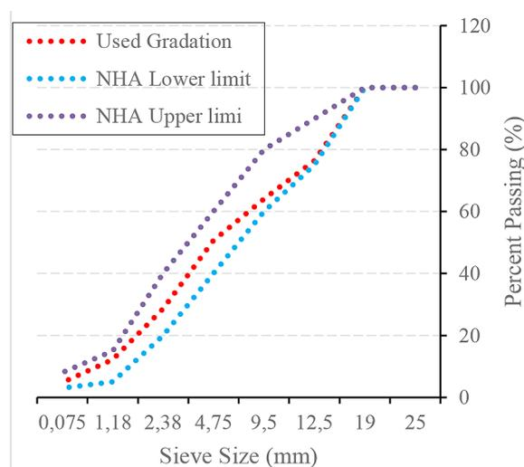
**Figure 5.** Blend gradation-1 for 3% filler
