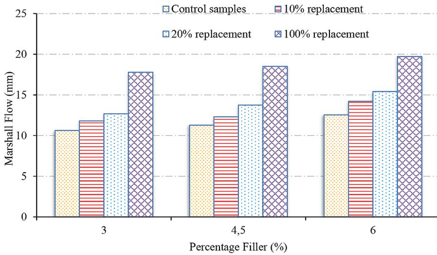
Figure 9. Marshall flow vs filler content for different replacements
