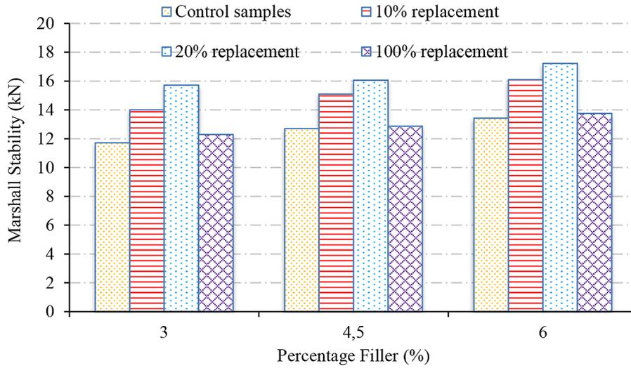
Figure 8. Marshall stability vs filler content for different replacements
