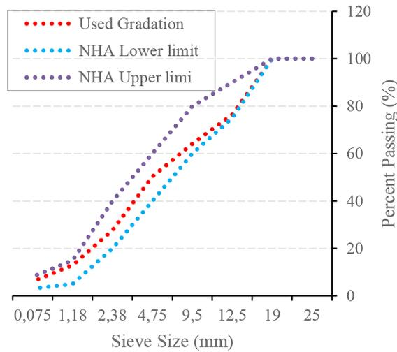
Figure 6. Blend gradation-2 for 4.5% filler
