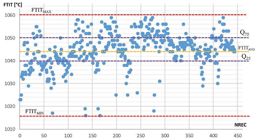
Figure 14. Example engine trending parameter FTIT not working on the FTIT limit
