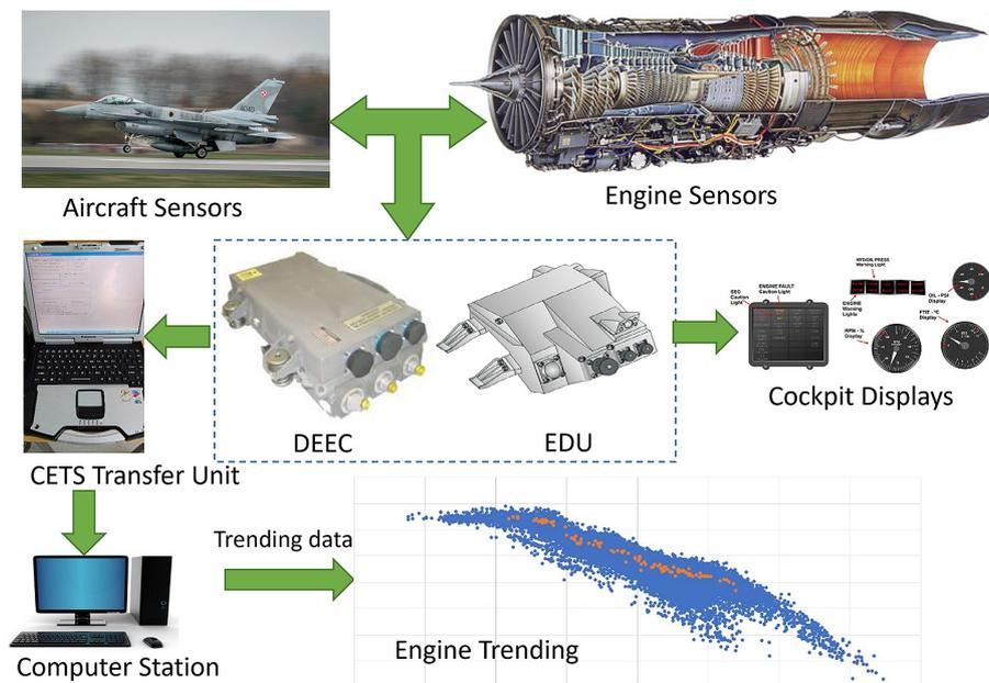
Figure 1. Engine monitoring system data flow
