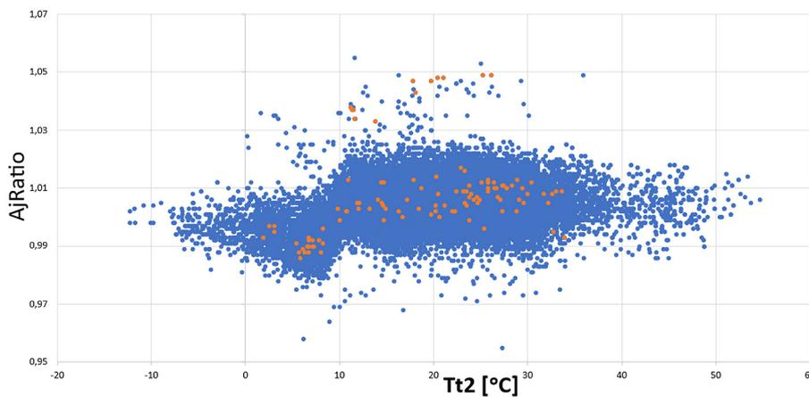
Figure 3. Engine life cycle trending Aj vs. Tt2
