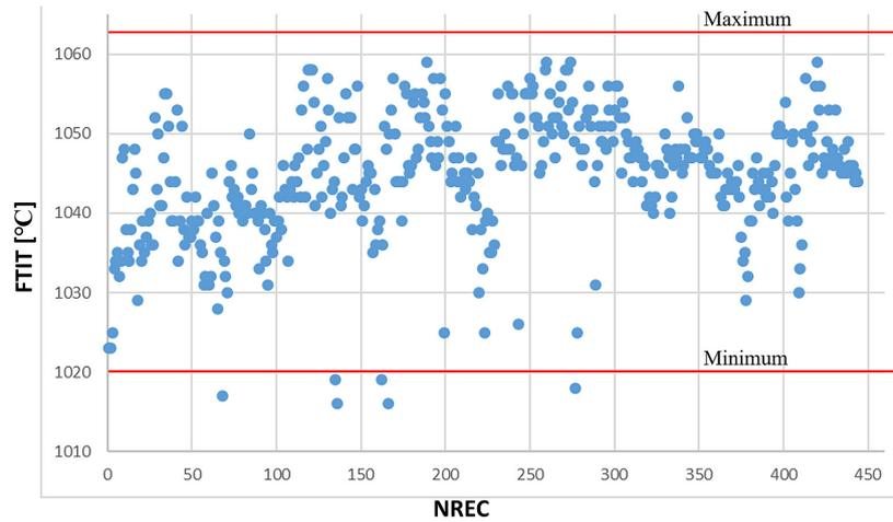
Figure 11. Engine data parameters trending absolute limit (AL)
