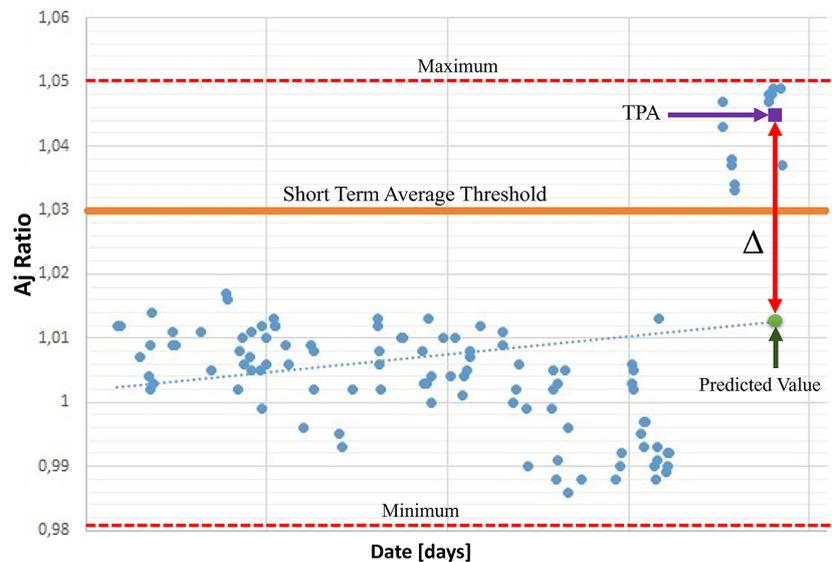
Figure 15. Engine data parameters trending  $A_j$  Ratio vs date
