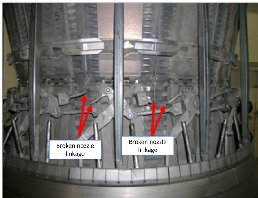
**Figure 16.** Engine nozzle crunch resulted in broken nozzle linkages
