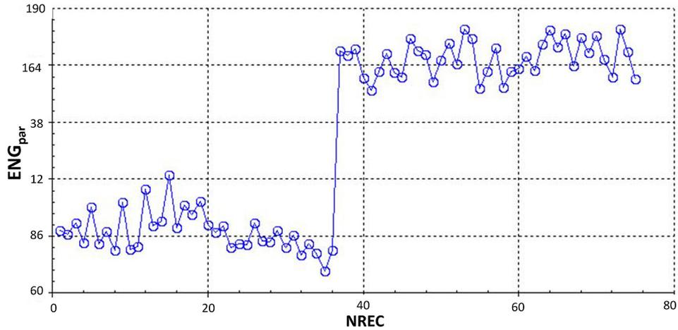
Figure 6. Engine parameter sudden step change
