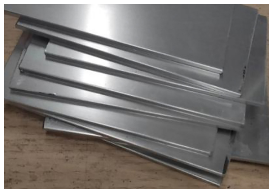
Figure 4. Aluminum plates onto which the paint coating was applied [17]
