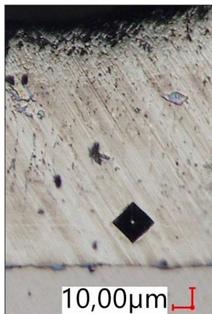
Figure 3. Methodology for measuring the microhardness of zinc coatings
