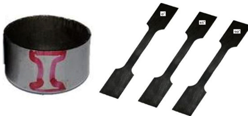
Figure 6. The tensile test specimens were taken from sheets of metal and cylindrical shapes according to ASTM standard E8M specification
