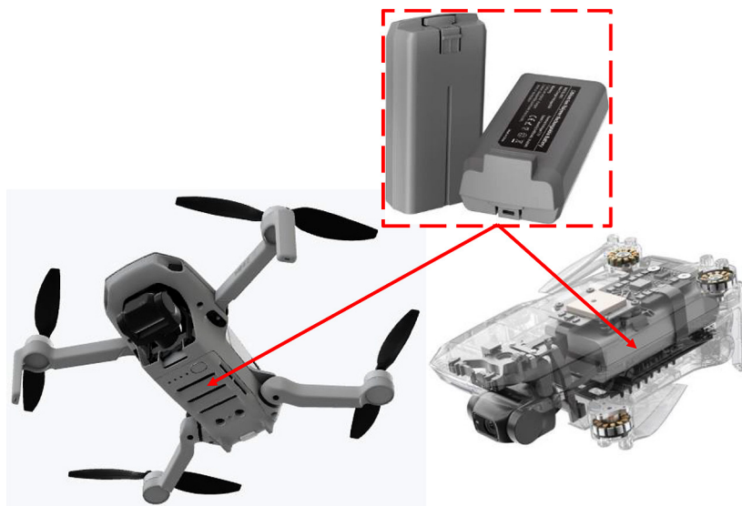
Figure 1. UAV platform used for in-flight experiments: DJI Mini Combo 2 and its battery location
