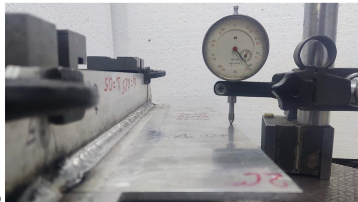
Figure 4. Measurements of residual welding displacements (deformations) in specimens of butt (a) and tee (b) welded joints
