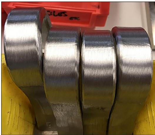
**Figure 6.** Weld's samples welded after the bend test
