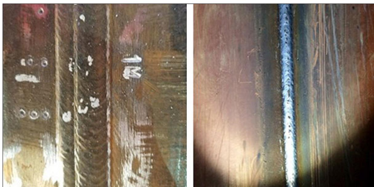
Figure 5. View of the weld from the face and the ridge
