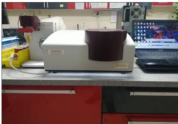
Figure 3. Zeta potential device
