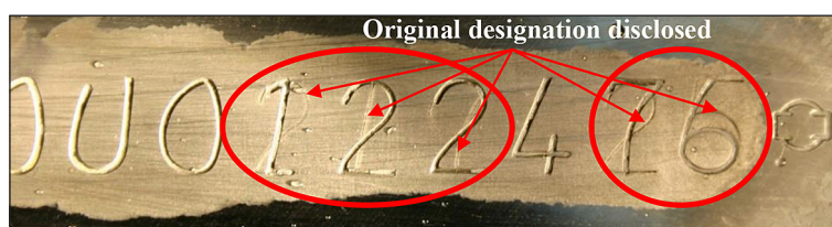
Figure 15. Fragment of a processed number field with the original labelling disclosed by the chemical method
