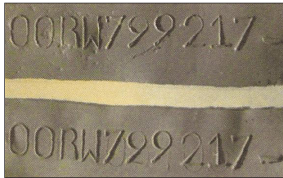
Figure 4. Silicone cast a numerical field made before research and after tests [12]
