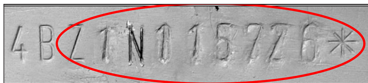
Figure 19. Part of the vehicle number field with visible changes to the marking
