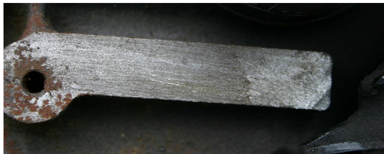
Figure 17. Number field with sanded off marking
