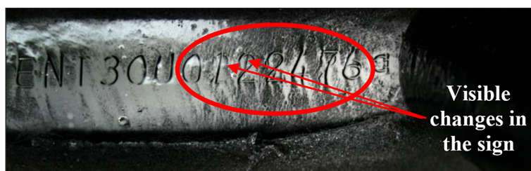
Figure 13. Displays changes in the number field using a constant magnetic flaw detector
