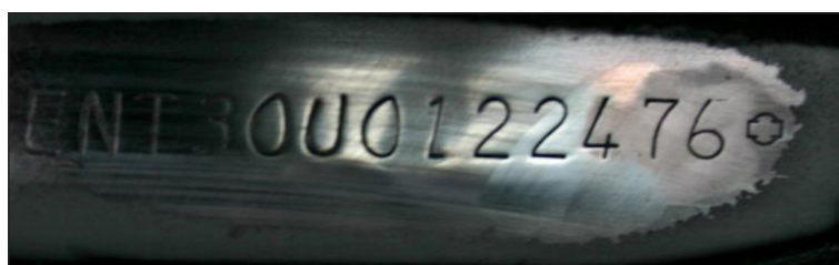
Figure 14. Number field after removing varnish and base paint
