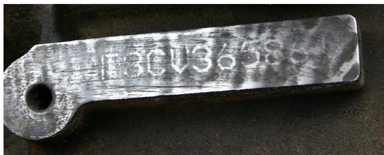
Figure 18. Revealed identification marking using the thermal method
