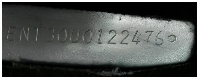
Figure 12. Numeric box made with punching method without visible changes
