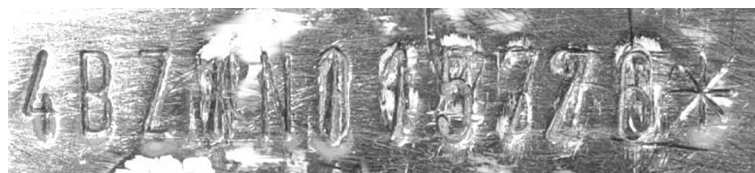
Figure 20. Primary VIN Marking Revealed
