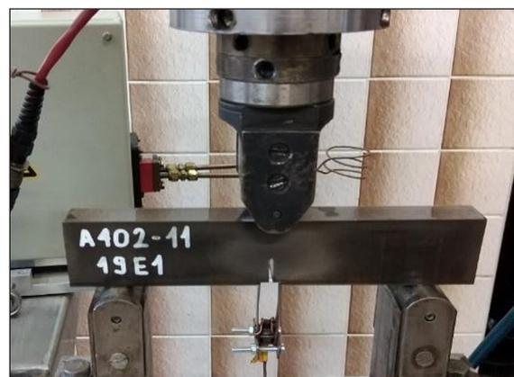
Figure 3. Generating a pre-fatigue crack
