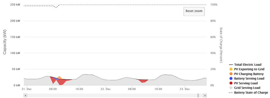
Figure 2. Operating schedules of local electrical network equipment when it connected to the network on December 22 (capacity of SPP is 163 kW)
