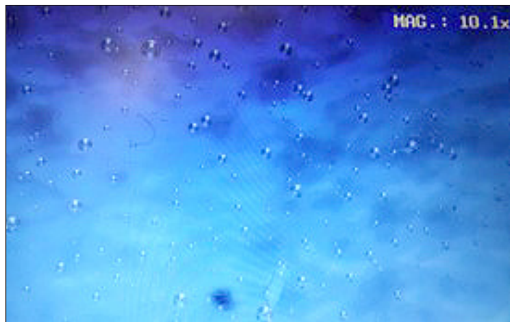
Figure 6. Resin composite (100:30) non-gasses – magnification 9.5×
