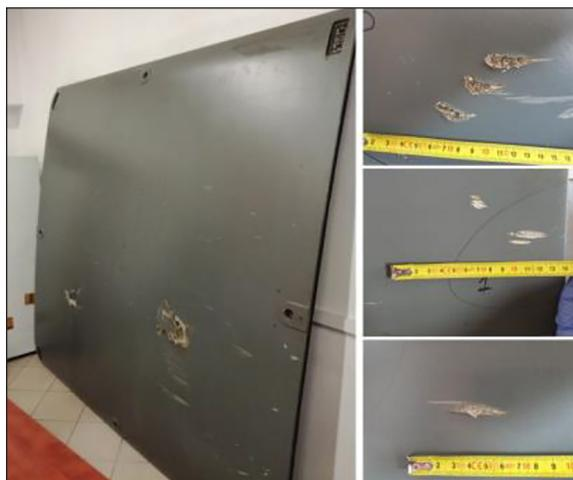
**Figure 3.** A cover from an electric multiple unit withdrawn from service due to multiple erosion damages and perforations. On the right side a detailed view of exemplary damage with dimensions
