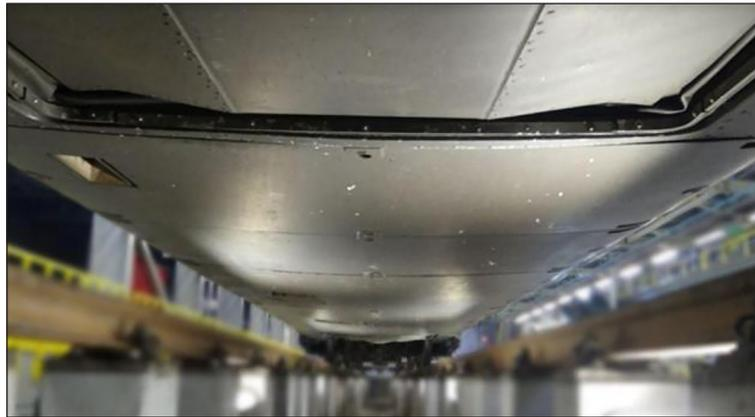
Figure 1. Chassis of a railway vehicle equipped with protective guards
