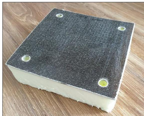
**Figure 8.** Composite sample with XPS core
