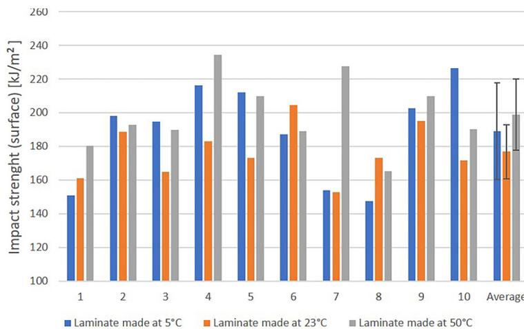
Figure 10. Impact strength of laminates under surface load
