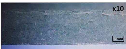
Figure 4. Internal structure of the composite made at 23 °C (x10 magnification)
