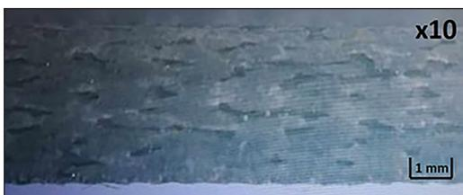
Figure 3. Internal structure of the laminate made at 5 °C (x10 magnification)
