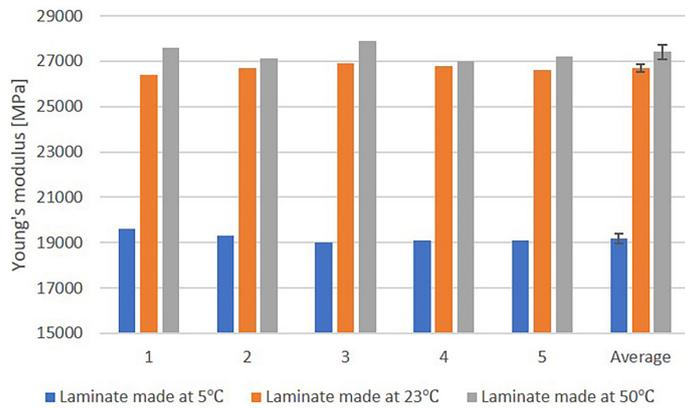
Figure 7. Diagram of Young's modulus (tensile) of tested materials
