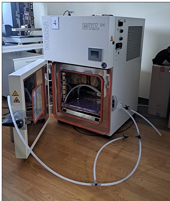
**Figure 1.** WEISS-Technik climate chamber WKL 64/40 including vacuum installation
