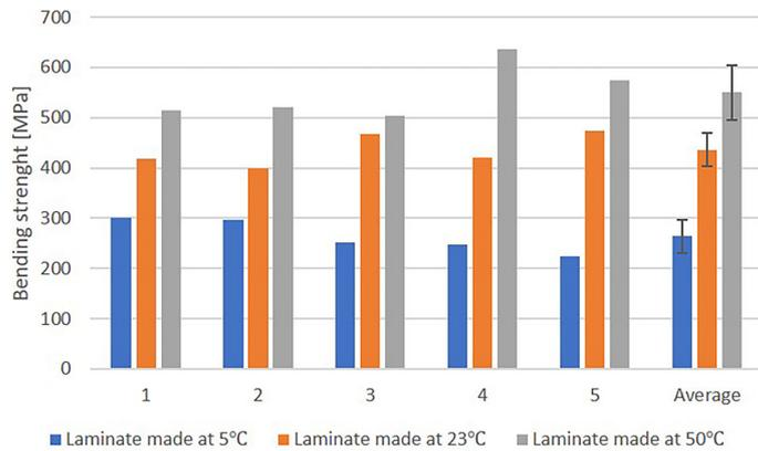
Figure 8. Diagram of the bending strength of the test materials
