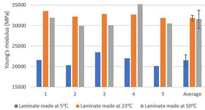
Figure 9. Diagram of Young's modulus (bending) of tested materials
