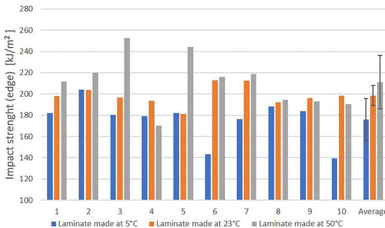
Figure 11. Impact strength of laminates under edge loading
