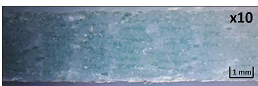
Figure 5. Internal structure of the composite made at 50 °C (x10 magnification)
