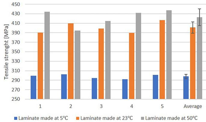
Figure 6. Diagram of tensile strength of tested materials
