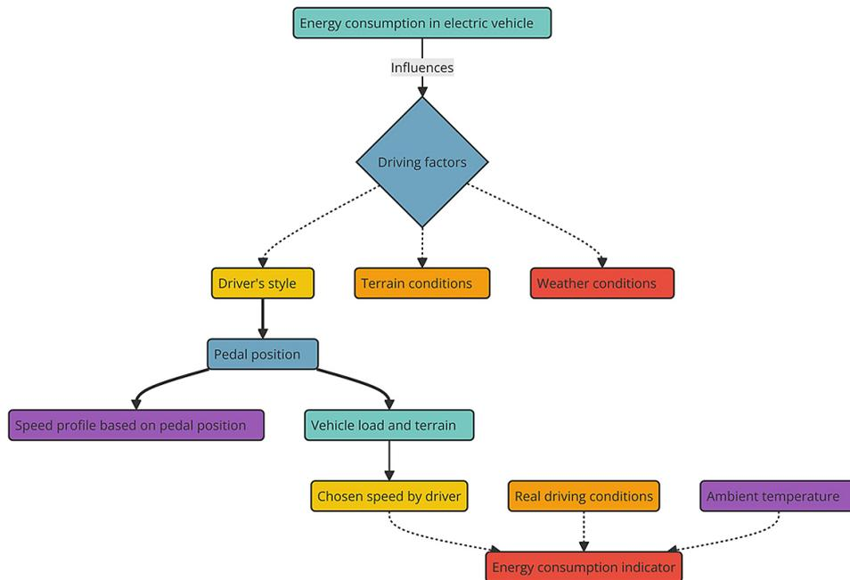
Figure 5. Relationships affecting energy consumption in an electric vehicle
