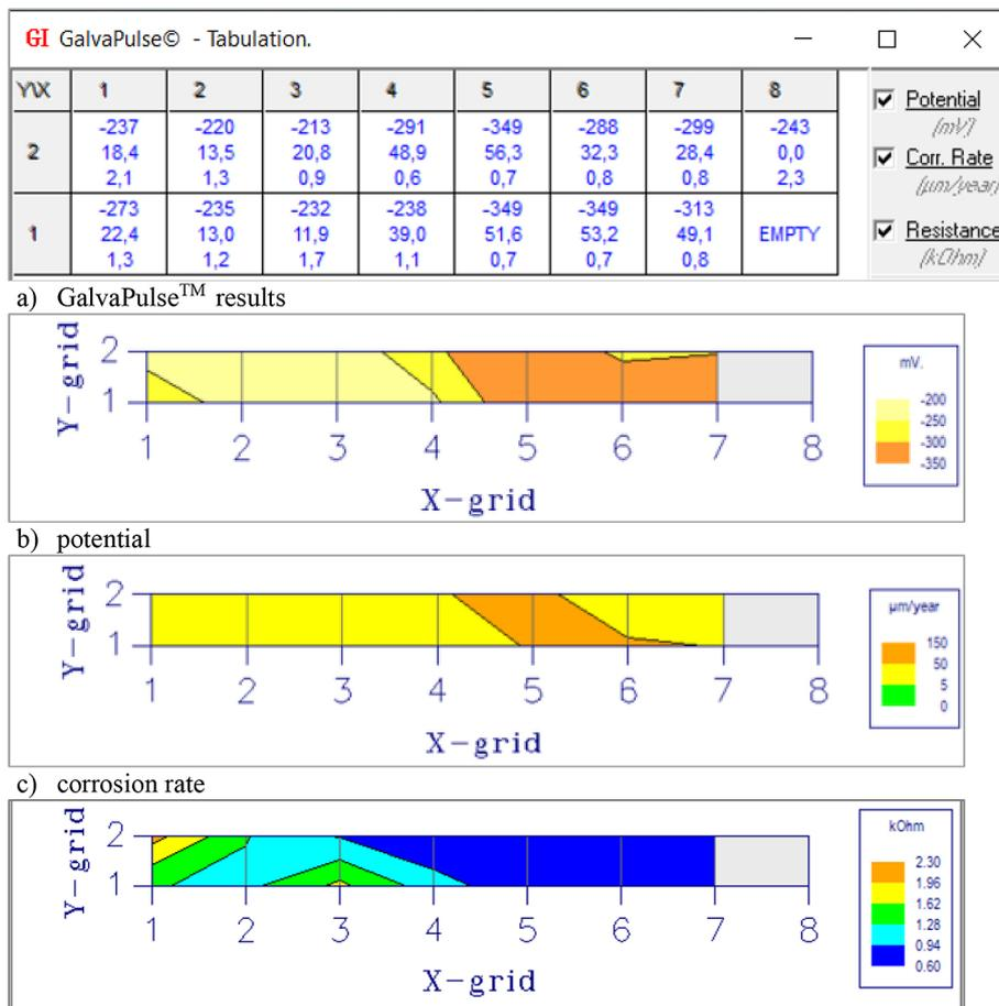
Figure 8. Results of the parameters measured by the GalvaPulse™ method: a) tabular summary, b) stationary potential of the reinforcement, c) corrosion current density, d) resistivity of the concrete cover
