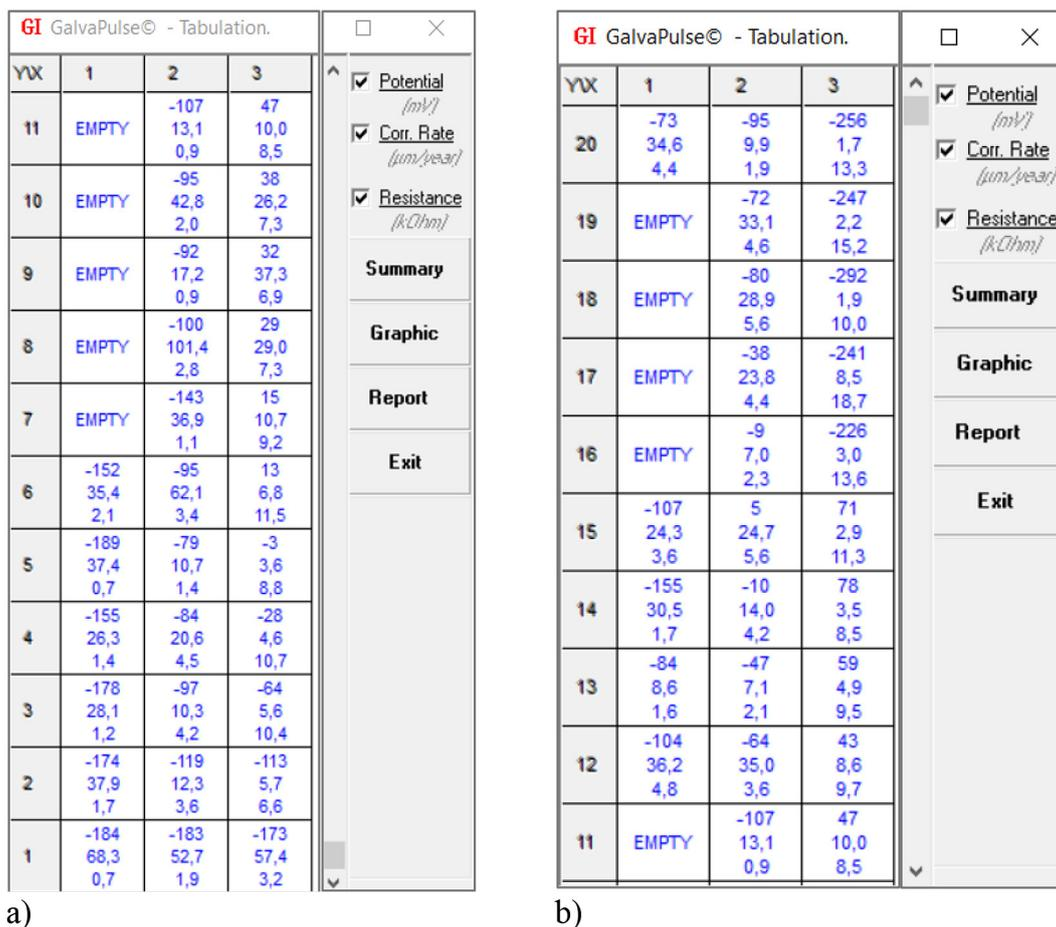
Figure 4. Table of results obtained by the GalvaPulse™ method [29]
