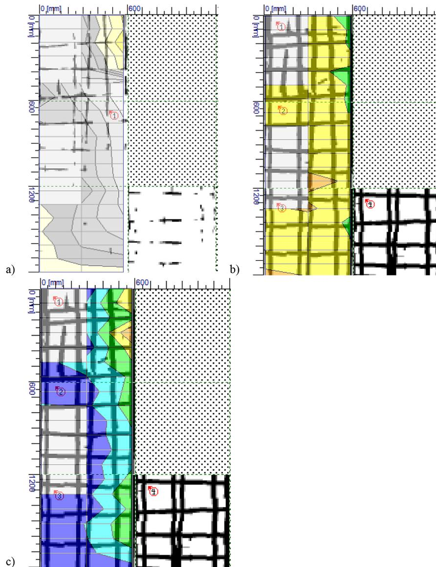
**Figure 3.** Images of the loggia wall reinforcement system with applied colour corrosion estimation maps and a table of results obtained by the GalvaPulse™ method: a) stationary potential of reinforcement, b) corrosion current density, c) resistivity of the concrete cover [29]
