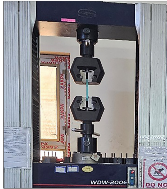
Figure 5. Universal Testing Machine WDW-200E examine the printed sample printed specimen
