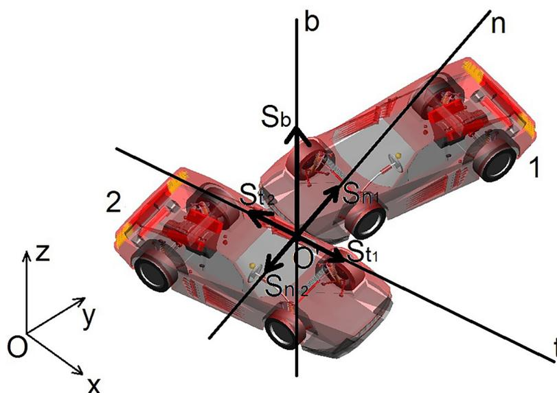
**Figure 1.** The location of both vehicles at the beginning of the collision with the components of the collision force impulse and the numbers of vehicles marked [based on 3]
