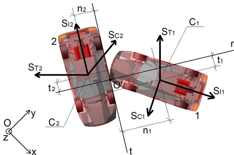
Figure 5. The impulses of the forces in resultant motion in a plan view [based on 3]
