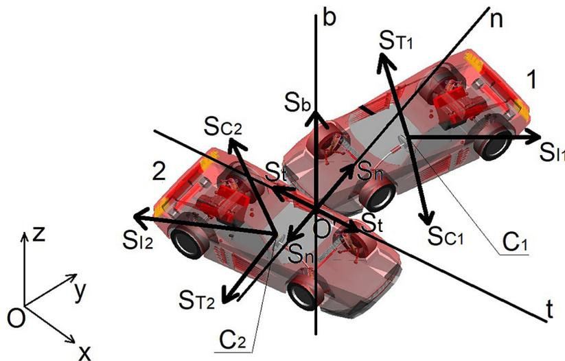
Figure 4. The impulses of the forces in resultant motion [based on 3]
