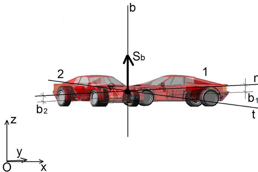
**Figure 3.** The physical model of the front, eccentric and oblique impact with the impulses of the impact force marked in a plan view [based on 3]
