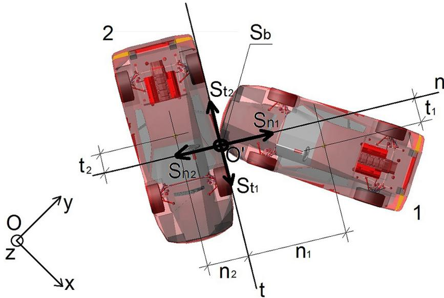
**Figure 2.** The physical model of the front, eccentric and oblique impact with the impulses of the impact force marked in a plan view [based on 3]
