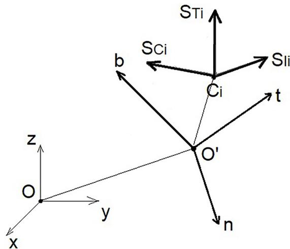
Figure 9. Mutual location of the impulses of forces in the resultant motion during the collision
