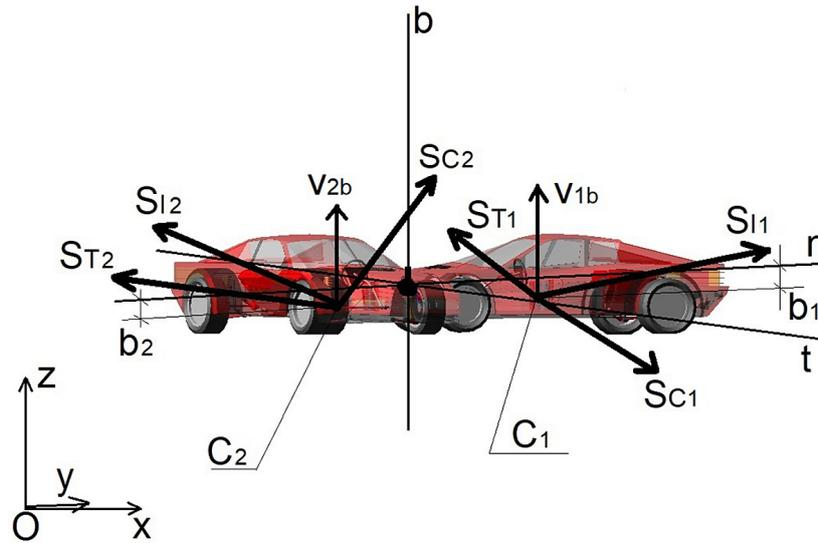
Figure 8. The components of the velocities of both vehicles in a side view [based on 3]
