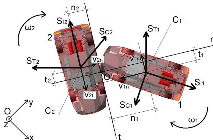
Figure 7. The components of the translational and the angular velocities of both vehicles in a plan view [based on 3]
