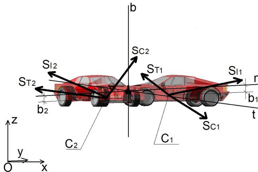
Figure 6. The impulses of the forces in resultant motion in a side view [based on 3]
