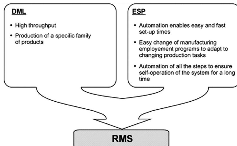
Fig. 1. Advantages of conventional manufacturing systems combined by the RMS
