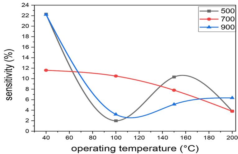
Figure 5. Sensitivity vs. operating temperature of  $\text{SiO}_2$ -NiO nanocomposite films at the specified temperatures for  $\text{NH}_3$  gas. The lines connecting experimental points are the ‘eye-guide’ only
