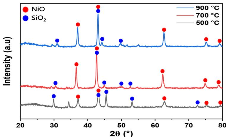
**Figure 1.** X-ray diffraction patterns of  $\text{SiO}_2$ - $\text{NiO}$  nanocomposite films at three calcination temperatures ( $500$ ,  $700$ ,  $900^\circ\text{C}$ ). Diffractograms were shifted arbitrarily for better visualization
