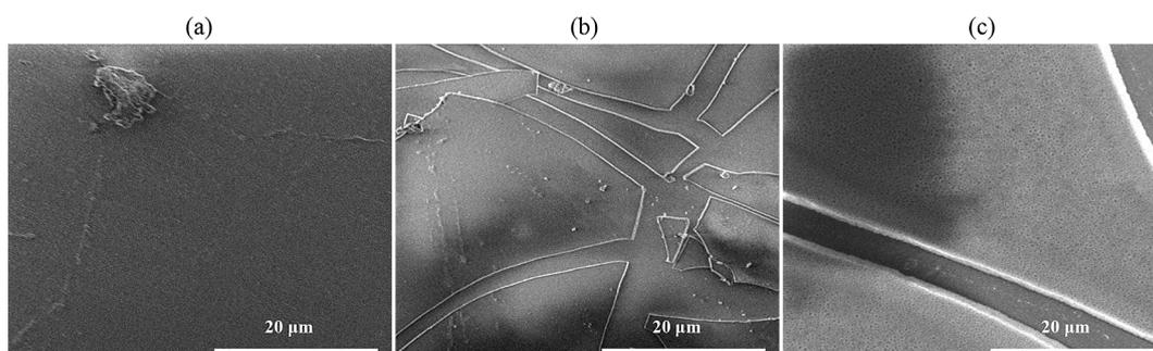
**Figure 2.** SEM images of  $\text{SiO}_2$ - $\text{NiO}$  nanocomposite films annealed at three temperatures: a)  $500^\circ\text{C}$ , b)  $700^\circ\text{C}$ , and c)  $900^\circ\text{C}$
