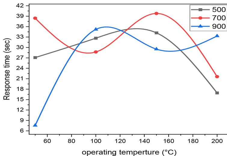
Figure 6. Response time of  $\text{SiO}_2$ -NiO thin films at different operating temperatures for  $\text{NH}_3$  gas. The lines connecting experimental points are the ‘eye-guide’ only
