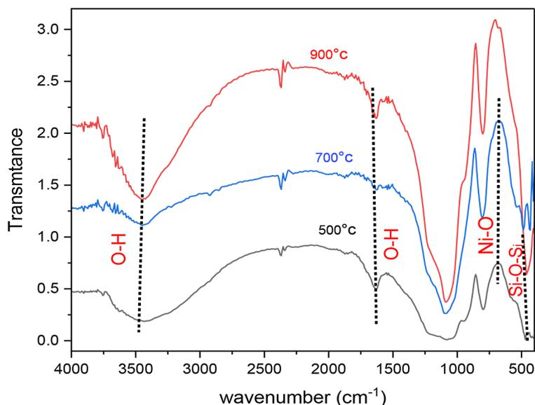
Figure 3. FTIR spectra of  $\text{SiO}_2\text{-NiO}$  nanocomposite films annealed at different temperatures
