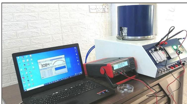
Figure 4. Gas sensing apparatus
