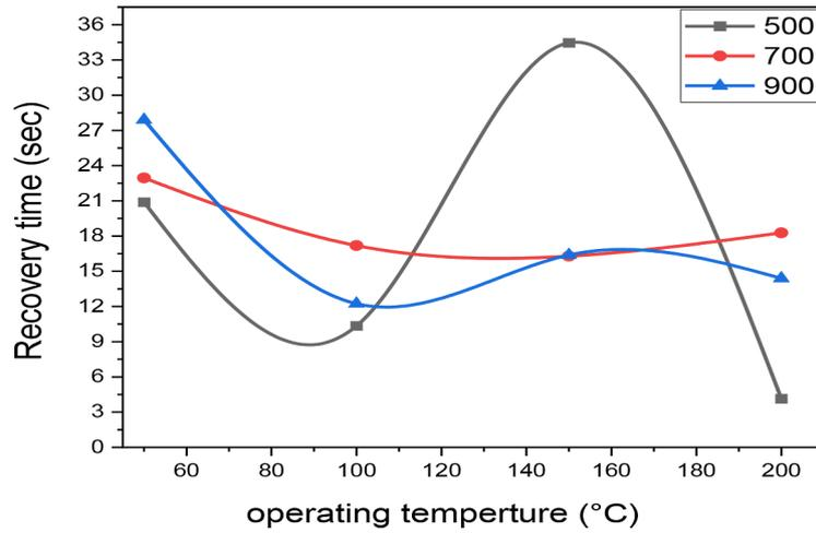
Figure 7. Recovery time of SiO<sub>2</sub>-NiO thin films at different operating temperatures for NH<sub>3</sub> gas. The lines connecting experimental points are the ‘eye-guide’ only
