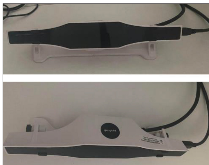
Figure 5. Structure of the GP3 eye tracker
