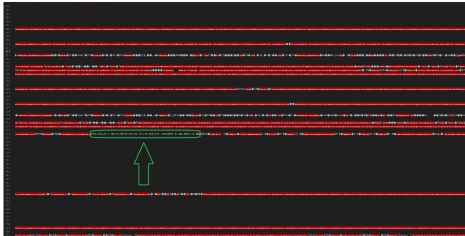
Figure 4. Hiding data in the file's metadata. The green arrow marks the area for entering data saved in open text
