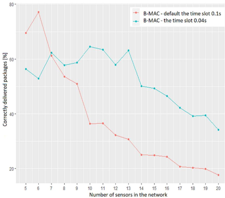
Figure 3. Packet delivery correctness simulation results for B-MAC protocol
