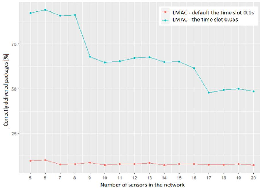
Figure 5. Packet delivery correctness simulation results for L-MAC protocol
