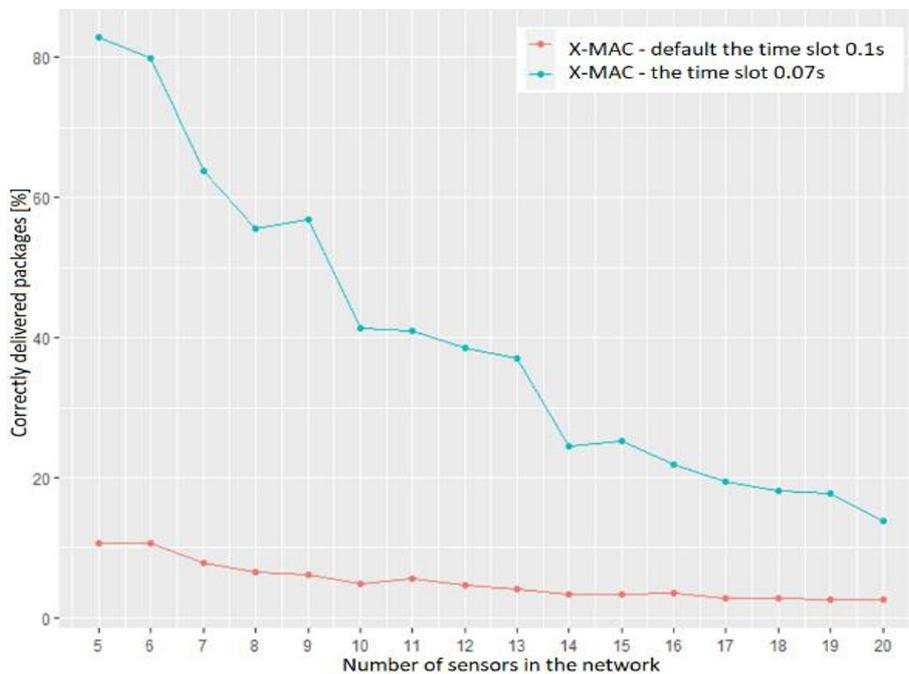
Figure 4. Packet delivery correctness simulation results for X-MAC protocol
