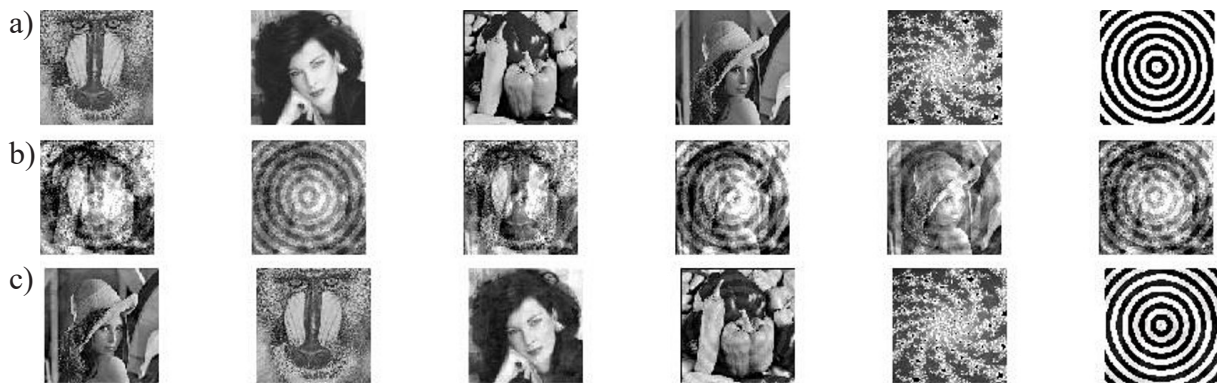
Figure 1. Separation results using four natural images of 128×128 pixels in size (a) original source images, (b) mixed images, (c) recovered sources using the proposed algorithm
