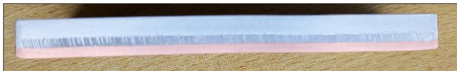
**Figure 2.** View of the composite sample after joining by explosive welding
