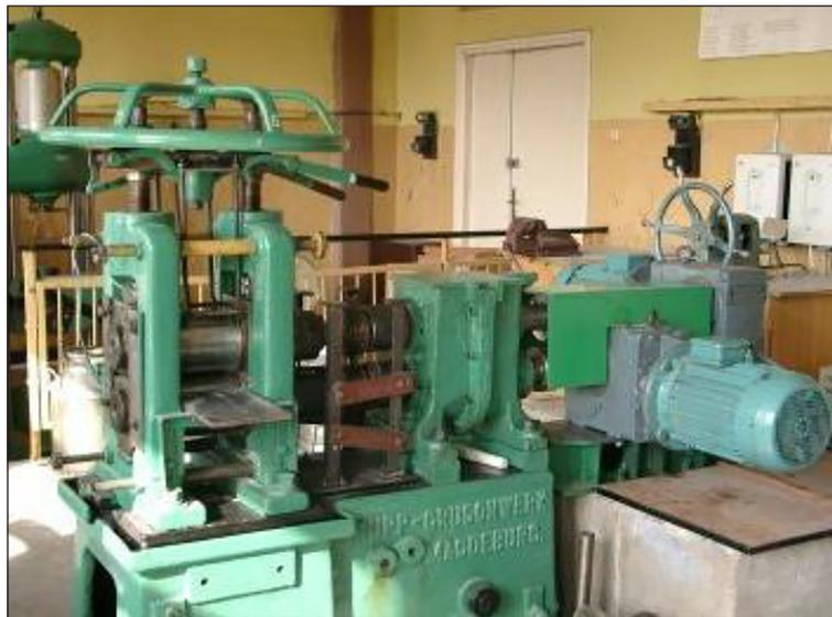
**Figure 3.** View of the duo rolling mill φ150 mm
